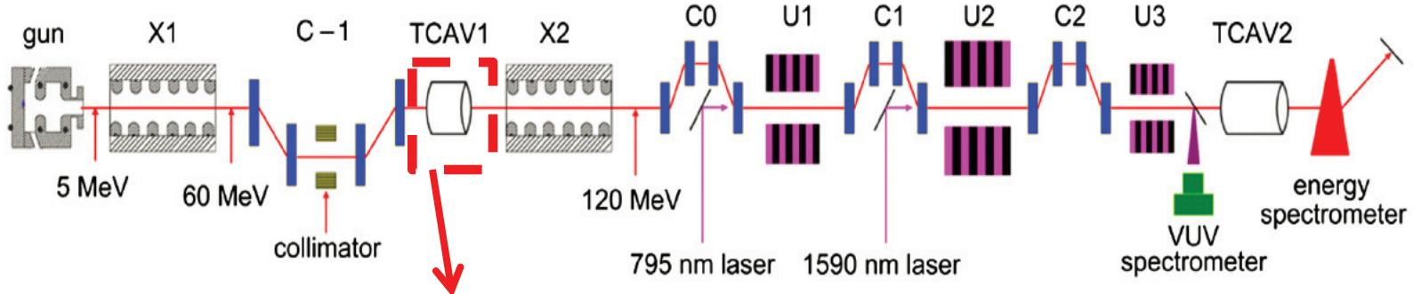
➤ In order to confirm the main advantage of EEHG over HGHG, a radio-frequency (RF) transverse cavity (TCAV1) is installed in the NLCTA beamline to increase the slice energy spread by 1 order of magnitude (works as a laser heater).
