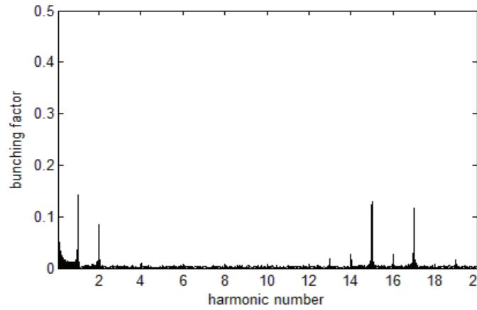
Remarkable up-frequency conversion efficiency:  $b_n \sim n^{-1/3}$  Fully coherent soft X-ray
