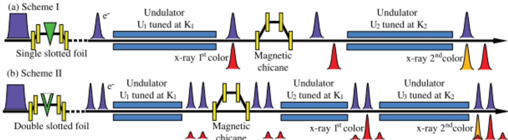
Two-color FEL schemes tested at the LCLS. A single-slot (in scheme I) or double-slot (in scheme II) emittance spoiling foil was used to generate ultrashort single or double electron bunches. The emittance-spoiling foil is located in the second bunch compressor. A magnetic chicane, designed for hard x-ray self-seeding purpose, was adopted here to control the temporal delay between the two-color pulses.
