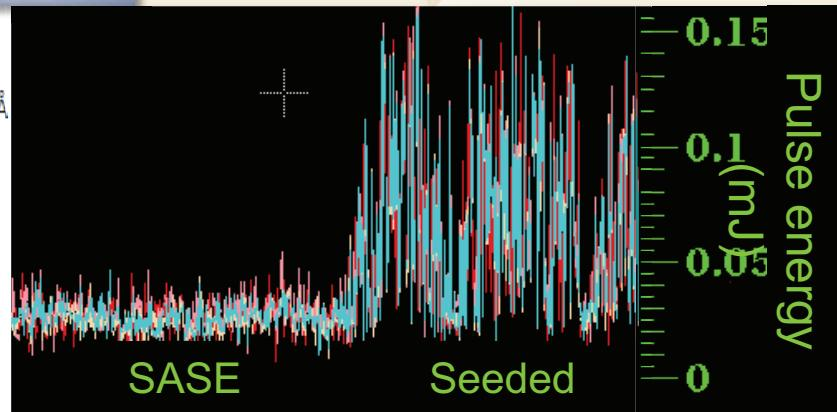
Single shot pulse energy from the gas detectors with 40pC charge
