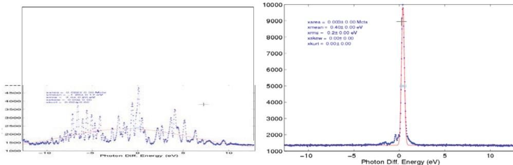
SASE and Seeded spectra recorded on single shots. The left panels are SASE with 150 pC, 3kA peak current, un-seeded. The FWHM of the SASE spectrum is 0.2 % Bandwidth. The right panels are the seeded beam with the same electron beam parameters. The FWHM of the seeded beam is 0.5 eV ( $5 \times 10^{-5}$  bandwidth)
