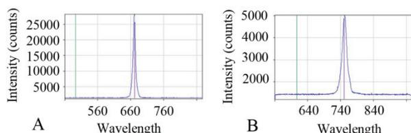
Figure 3: Spectral energy distribution of the LEBRA-FELs with peak emission at 660 nm (A) and 740 nm (B).
