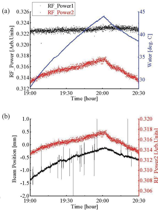
Figure 6: RF input power relative to (a) cooling water or (b) beam position at BPM#2.
