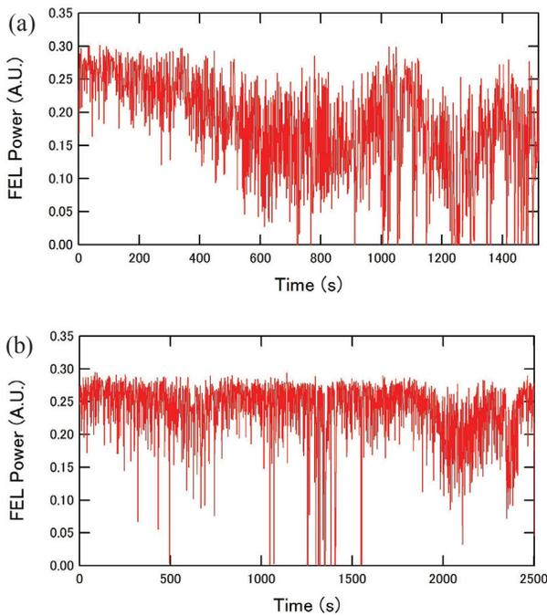
Figure 2: The fluctuation of FEL Power (a)without feedback control (b)with feedback control[1].
