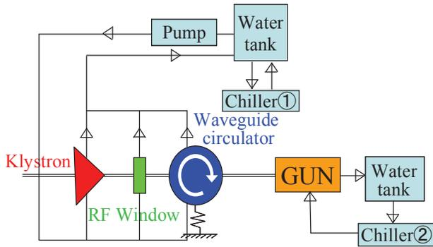
Figure 5: Circulation route of cooling water.
