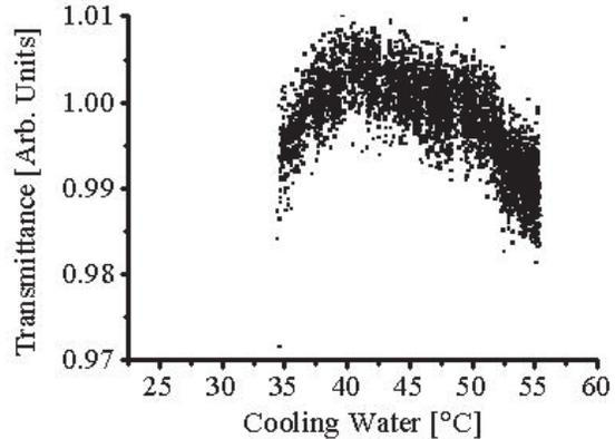
Figure 7: Optimum temperature of water for cooling circulator.
