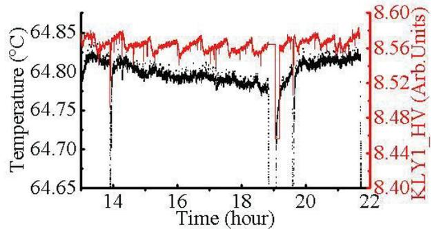
Figure 3: Effect of Cavity temperature on beam energy.
