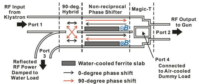
Figure 8: Structure of 4-port waveguide circulator.
