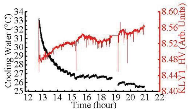
Figure 4: Relation between Cooling Water and Klystron High voltage.
