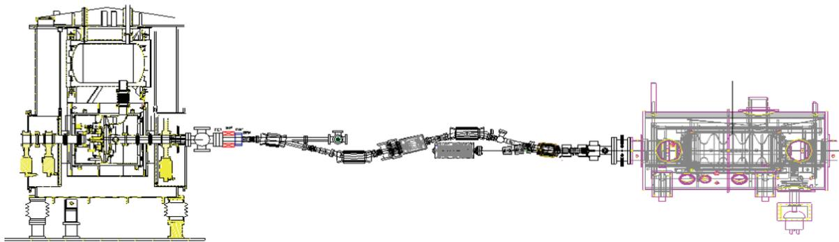
Figure 2: Detailed drawing of SRF Injector for the BNL R&D ERL.
