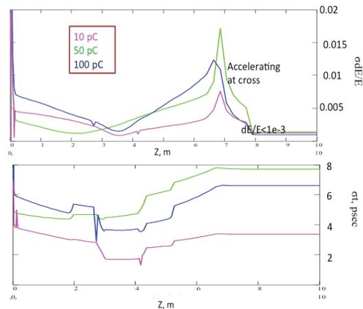
Figure 6: Longitudinal beam dynamics for low charge operation: Evolution of energy spread (top figure – rms energy spread, bottom figure- rms bunch length) in the ERL injector. Bunch charge: 10 pC -magenta, 50 pC - green, 100pC –blue.)
