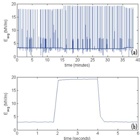
Figure 4: 5 cell cavity performance during horizontal test. Pulses are 2 seconds long with a 30 second interval.
