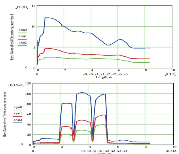
Figure 5: Evolution of normalized beam emittances in ERL injector (top figure – horizontal, bottom figure-vertical). Bunch charge: 0.7 nC-GREEN, 1.4 nC- RED, 5nC –BLUE.
