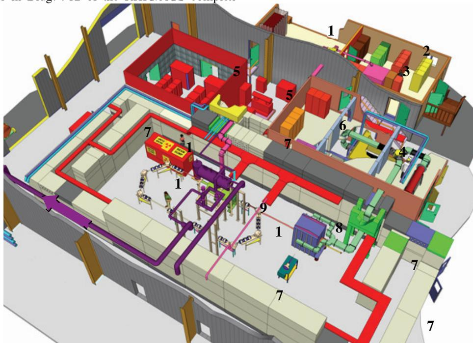
Figure 1: Layout of the R&D energy recovery linac in the shielded vault in bldg 912: 1-Control Room; 2-diagnostic and control racks; 3-704 MHz 50 kW CW RF transmitter; 4- 704 MHz 1MW CW klystron; 5- 2MW CW HV power supply for the klystron; 6- magnets power supplies and other controls; 7-shielded ERL vault with removable beams; 8- 2 MeV 704 MHz SRF photo-injector; 9- 15-20 MeV 704MHz 5-cell SRF linac; 10 -return loop; 11- beam dump.
