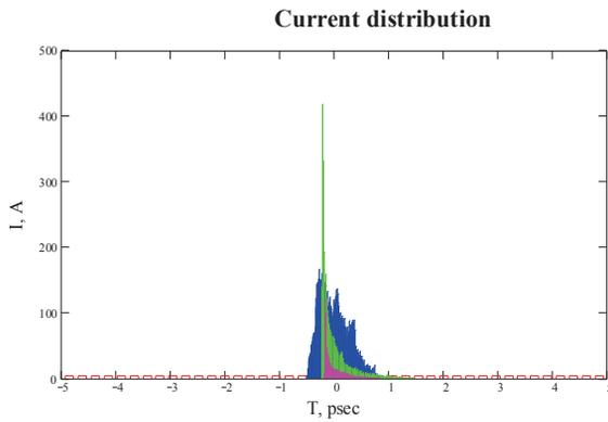
Figure 7: Current distribution after compression: magenta Q=10 pC,  $\sigma_z=59\mu\text{m}$ ,  $I_{\text{max}}=120\text{ A}$ , green Q=50 pC,  $\sigma_z=89\mu\text{m}$ ,  $I_{\text{max}}=418\text{ A}$ , blue Q=100 pC,  $\sigma_z=83\mu\text{m}$ ,  $I_{\text{max}}=167\text{ A}$ .
