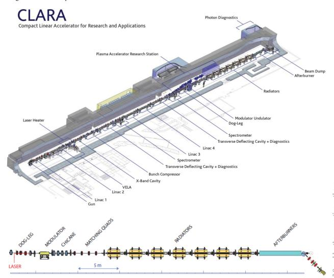
Figure 1: 3D Engineering representation of the CLARA facility (top) and enlarged 2D representation of the FEI systems (bottom).
