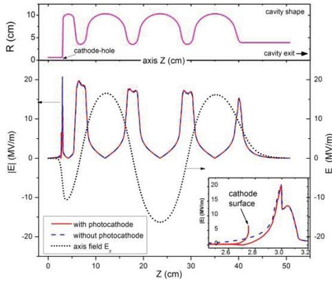
Figure 2: (Top) The cavity shape of ELBE SRF gun. (Down) The distribution of the electric surface field and the axis field, simulated using Superfish with  $E_{acc} = 6$  MV/m. (Inset) The distribution of the electric surface field in the zone closed to the cathode.
