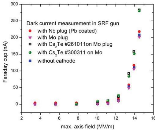
Figure 3: The dark current from the SRF gun.
