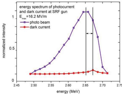
Figure 6: The energy comparison of the photoelectron beam and the dark current beam.
