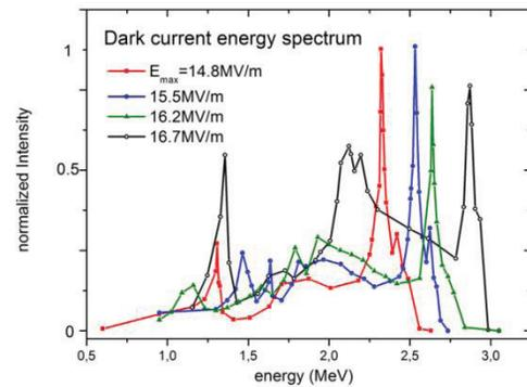
Figure 5: Energy spectra of the dark current of the SRF gun with a Mo photocathode.
