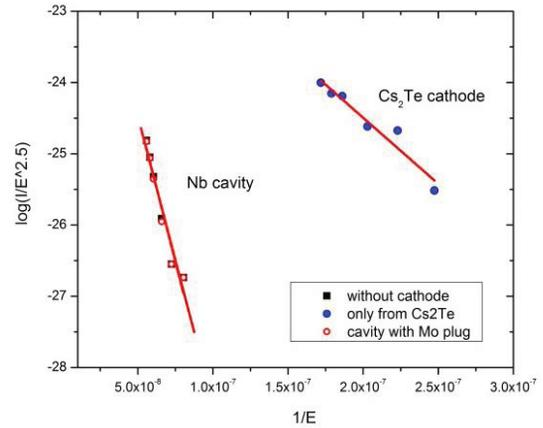
Figure 4: The graphical presentation of the measurement data in the way of Fowler-Nordheim plot.
