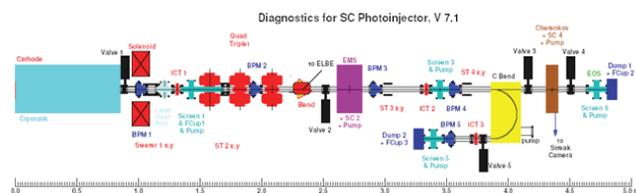
Figure 1: The diagnostic beam line for SRF gun. [8]
