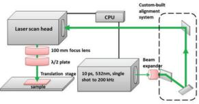
Figure 1: Ultra-short Laser configuration for materials processing.
