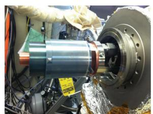
Figure 9: Photograph of the cathode stalk with copper cathode mounted on the transport cart.
