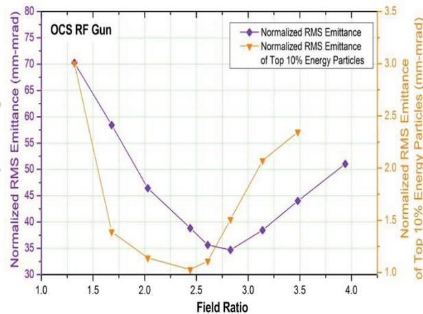
Figure 3: Dependence of the projected transverse emittance (purple) and the emittance of the electrons within the top 10% in energy (orange) on field ratio.
