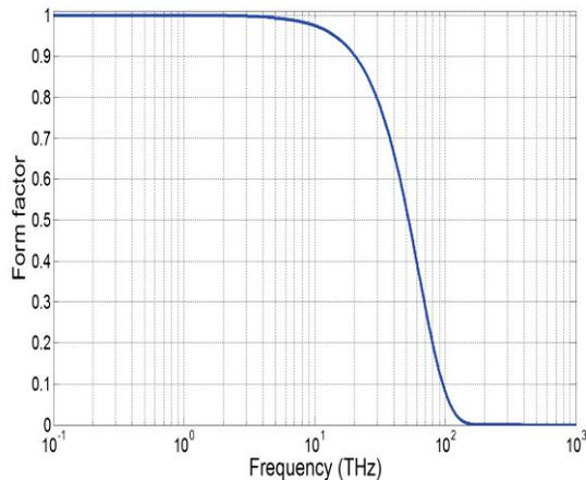
Figure 5: Bunch form factor of a 100 fsec beam as a function of THz frequency.
