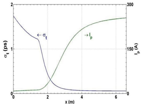
Figure 4: Evolution of the duration (blue) and peak current (green) of a 30 pC electron bunch along beam path from the alpha magnet exit to the 5.2 m linac exit. The accelerating gradient of the rf linac is set at 15 MV/m.
