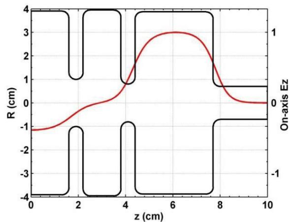
Figure 1: Geometry of the NSRRC 2998 MHz OCS rf gun. The red line is the relative amplitude of the longitudinal component of the rf electric field along the cavity axis when it is operated at  $\pi/2$ -mode.
