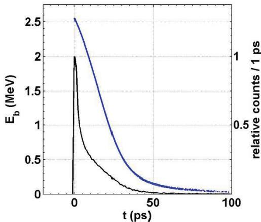
Figure 2: The Electron distribution in longitudinal phase space (blue) and the electron population in a bunch as a function of time (black) at operating field strength.
