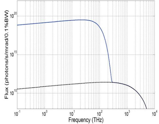
Figure 6: Spectrum of coherent synchrotron radiation in flux (blue). Incoherent synchrotron radiation (dashed line).
