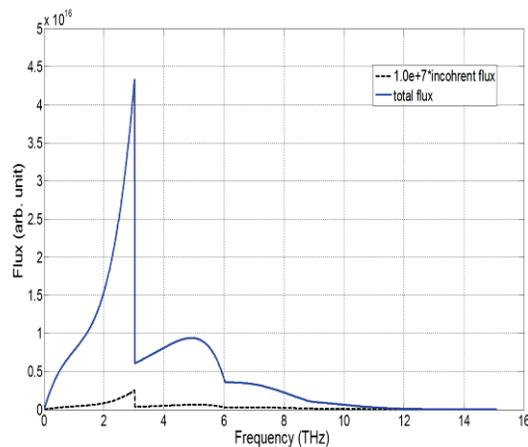
Figure 7: Spectral distribution of THz radiation energy from the 8 cm period helical undulator (blue). Incoherent undulator radiation spectrum is multiplied by a factor of 10,000,000 is also plotted for comparison purpose (dashed black).
