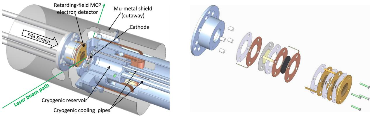
Figure 1: Detail of the TESS experimental system. **Left:** Overview with the vacuum chamber removed and the mu-metal magnetic shield and cathode holder cut away to aid clarity. The cathode holder is to the right, the detector to the left. **Right:** Schematic showing an exploded view of the retarding-field electron detector.
