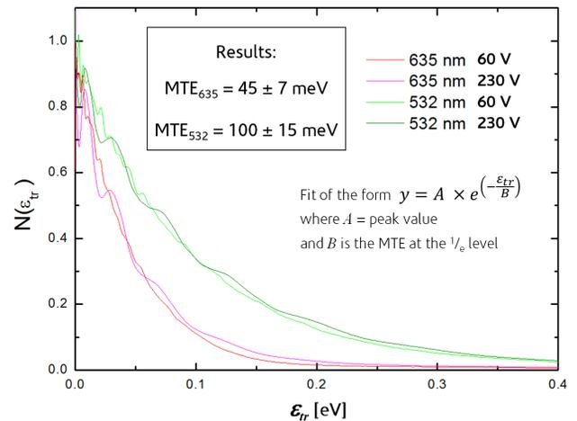
Figure 3: Measurements of transverse energy distribution curve and corresponding MTE for photoelectrons emitted from GaAs under illumination by red and green laser light.
