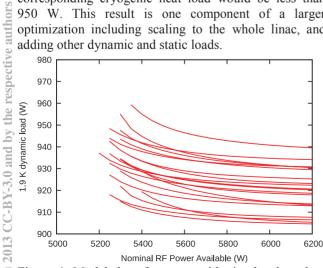
$\odot$  Figure 4: Modeled performance with simulated random  $\Xi$  production run of 112 cavities.
