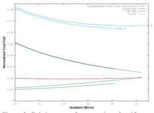
Figure 5: Relative cost of construction plus 15 years operation, as a function of cavity gradient. Operating cost assume 8000 hours per year, and \$0.12 per kW-hr.
