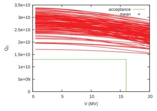
Figure 3: A simulated production run of 112 cavities. The green line shows the assumed acceptance criteria.
