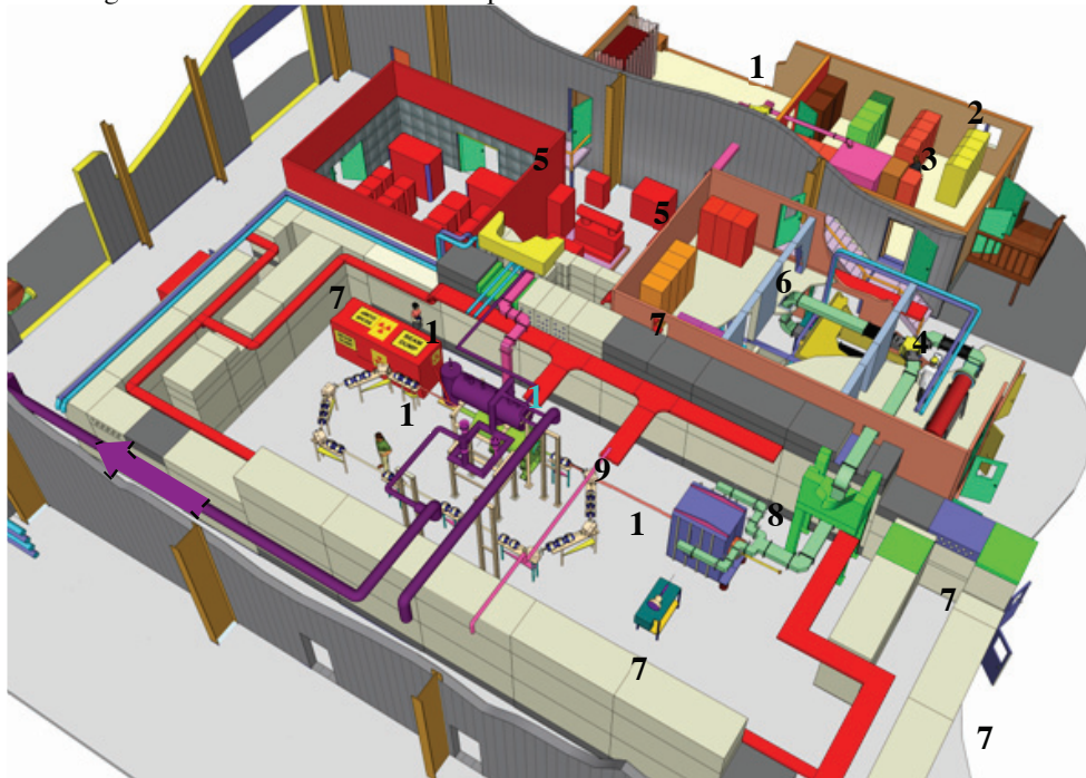
Figure 1: Layout of the R&D energy recovery linac in the shielded vault in bldg 912: 1-Control Room; 2-diagnostic and control racks; 3-704 MHz 50 kW CW RF transmitter; 4- 704 MHz 1MW CW klystron; 5- 2MW CW HV power supply for the klystron; 6- magnets power supplies and other controls; 7-shielded ERL vault with removable beams; 8- 2 MeV 704 MHz SRF photo-injector; 9- 15-20 MeV 704MHz 5-cell SRF linac; 10 -return loop; 11- beam dump.
