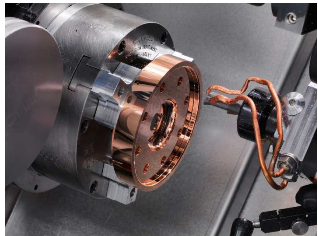
Figure 1: Copper cup in chuck of slant bed lathe after machining with monocrystalline tool.
