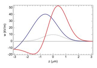
Figure 5: Wake of a Gaussian bunch with Q = 10 pC. The red line is computed with the singular Green function (5) and the blue line is computed with the new Green function (9). The dashed line shows the Gaussian bunch profile with the bunch head on the right.
