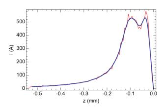
Figure 6: Beam profile at NGLS used for calculation of the wake. The red curve shows the original simulation, and the blue curve is a smoothed profile used for calculation of the wakes. The head of the bunch is on the right.
