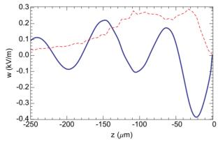
Figure 7: Wakefield for h = 100 nm. The red dashed curve shows the beam profile.
