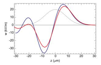
Figure 4: Wake of a Gaussian bunch with Q = 200 pC. The red line is computed with the singular Green function (3) and the blue line is computed with the new Green function (9). The dashed line shows the Gaussian bunch profile with the bunch head on the right.
