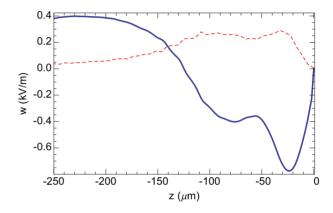
Figure 9: Wakefield for h = 500 nm. The red dashed curve shows the beam profile.
