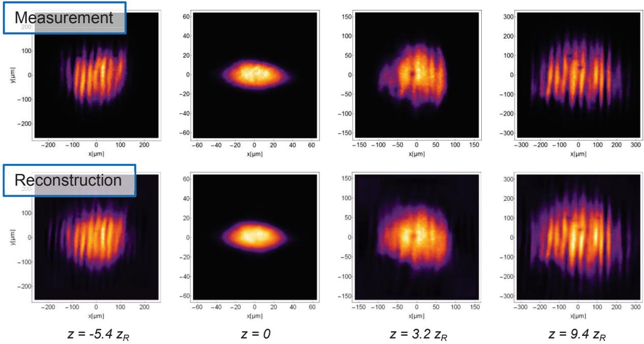
Figure 2: Normalized beam profiles at exemplary positions of the caustic. The upper row displays experimental data while the lower row shows reconstructed data from the Wigner distribution function.
