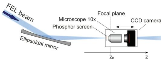
Figure 1: Experimental setup for caustic scan of the FLASH beam at BL2.
