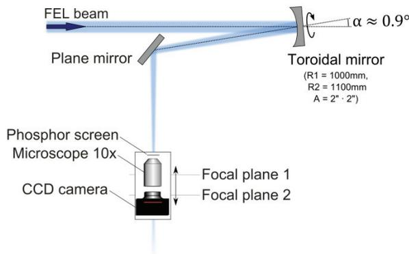
Figure 5: Extended experimental setup with toroidal mirror for four-dimensional phase space scanning.
