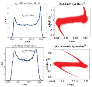
Figure 9: The bunch profile and phase space of low energy beam (top) and high energy beam before the undulator for 150pC beam. Bunch head is on the left.
