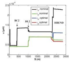
Figure 13: The growth of emittance along the hard X-ray beam line with 250 pC beam.
