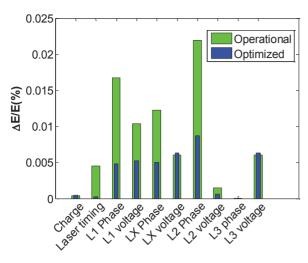
Figure 3: Comparison of the distribution of energy jitters for the operational mode and optimized one.
