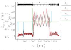
Figure 11: Twiss functions and dispersion along the Hard X-Ray beam line.
