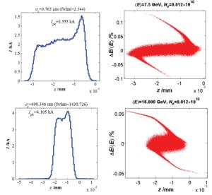
Figure 10. The bunch profile and phase space of low energy beam (top) and high energy beam before the undulator for 20pC beam
