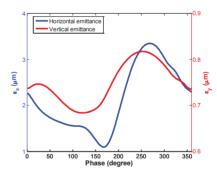
Figure 12: Effect of phase shift on the emittace at the beginning of the Undulator for 250pC Hard X-ray beam.
