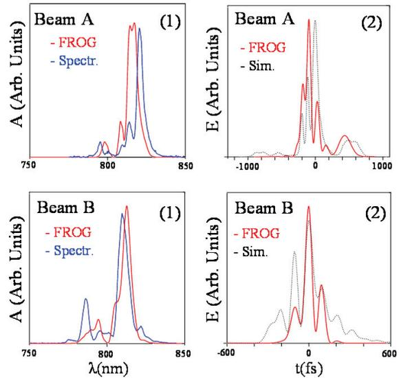
Figure 3: First row, beam A: panel (1) spectrometer signal (blue curve, abscissa on the top scale) and FROG spectral signal A (red curve, abscissa on the bottom scale). Panel (2): temporal pulse E from FROG (blue curve) and start to end simulation by Tstep and GENESIS 1.3 (black dotted curve). Second row: the same but for beam B.
