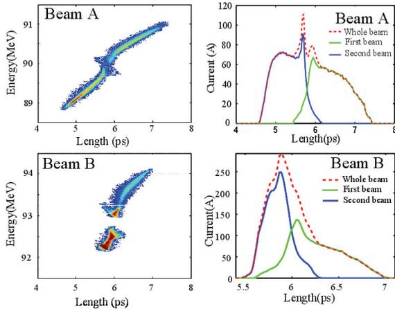
Figure 2: First row: Experimental electron phase space (1A) and electron current (2A) in the case of beam (A). Second row: the same for beam (B).
