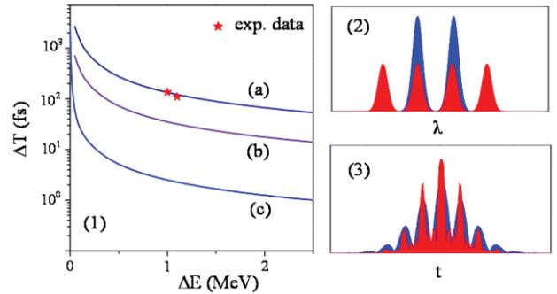
Figure 1: (1) Dependence of the fringe separation on the energy distance between the electron packets for (a) SPARC case,  $\lambda=800$  nm, (b)  $\lambda=30$ nm, (c)  $\lambda=0.15$  nm. Sketch of the spectrum (2) and temporal shape (3) of the pulse for  $N=2$  electron packets (blue curve) and  $N=4$  (red curve). The width of the fringes scales as  $1/N$ .
