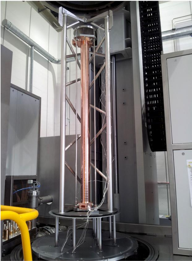
Figure 5: First 2 m long PSI C-band structure after the brazing.
