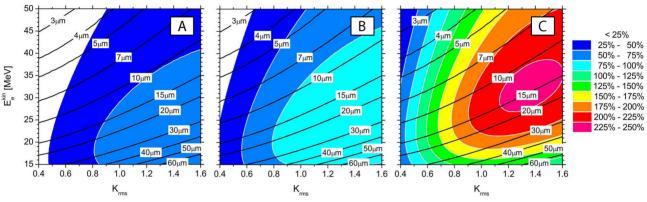
Figure 5: Single-pass small-signal gain calculated for three electron bunch lengths (rms) of (A) 5 ps, (B) 3 ps, and (C) 1 ps. In the calculation a bunch charge of 200 pC, an energy spread of 50 keV, and a normalized transverse emittance of 20  $\pi$  mm mrad have been assumed.
