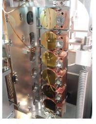
Figure 3: IR cavity mirrors for hole-outcoupling. Goldplated copper mirrors, with different diameters of the outcoupling hole are mounted on a precision translations stage (design by Bestec GmbH, Berlin). The 50-mmdiameter mirrors have a concave spherical surface of 3.51 m radius of curvature.
