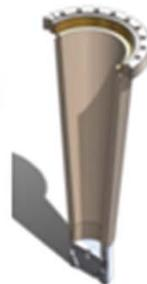
Cut-out of ball cathode design
