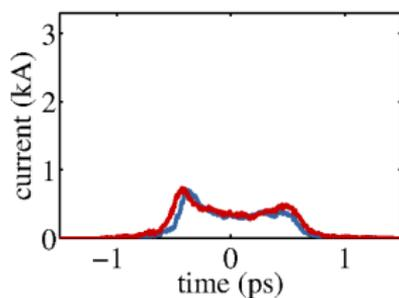
★ Local COTR emission spoils current profile measurement in non-dispersive section
