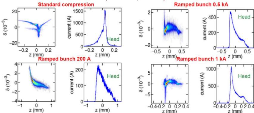
★ Linearly ramped current profiles (from experiment) enables (from simulations)  $R > 6$
