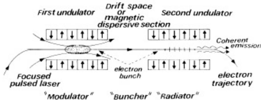
An **external laser is** focused in the “modulator”, which results in an energy modulation. It produces a density modulation in the dispersive section. Due to its anharmonicity, the laser harmonic frequencies are amplified in the radiator. This effect allows to produced **short wavelengths** at a **lower electron energy**.
