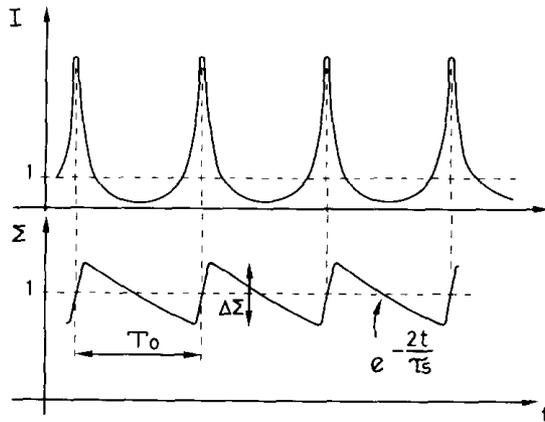
Fig. 3. Dimensionless laser intensity and energy spread in a pulsed storage ring free electron laser
