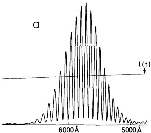
Fig. 3. Spontaneous emission spectrum  $dI/d\lambda d\Omega$  measured for an electron energy of 238 MeV and a magnetic field parameter of  $K = 2.09$  at low current where the modulation is almost total. The current decay  $I(t)$  is superimposed
