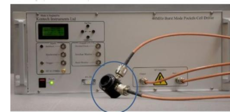
Burst mode Pockels cell mounted on optical table
