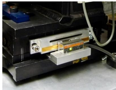
Encoder for relative cavity length measurement
