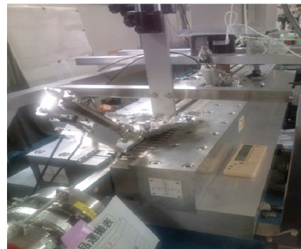
Figure 2: Hybrid-type 1.8-m undulator.
