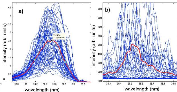
Figure 4: (a) Single-shot spectra of the SASE-radiation. (b) Single-shot spectra of the HHG-seed. The red curve is the average over all single shots.
