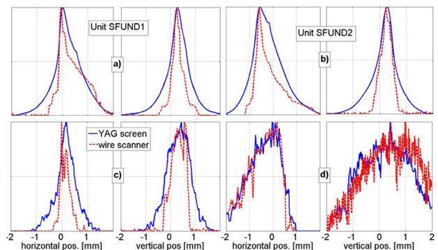
Figure 3: Electron beam profiles (upper row a) and b)) and XUV-laser beam profiles (lower row c) and d)) each measured with cerium-doped YAG screens and EMCCD cameras (blue lines) and with wire scanners (red lines) after adjusting the transverse laser position. The profile intensity is normalized to the same peak value for each measurement.
