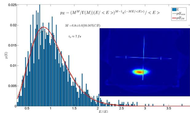
Figure 5: Probability distribution of the energy in the SASE-pulses and transverse profile of the SASE radiation on the YAG screen (inset).
