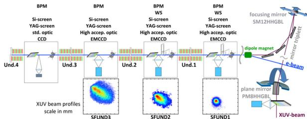
Figure 2: The schematic of the sFLASH beamline. It illustrates the injection beamline for the seed laser and the beam diagnostic stations. Exemplary XUV beam profiles along the undulator using a mirror with a focal length of 6.25 m [3].
