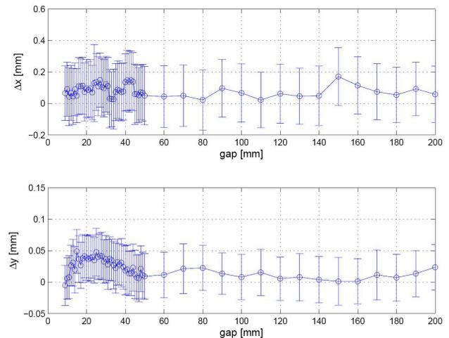
Figure 1: Electron beam position as a function of the gap of the first sFLASH-undulator at a BPM downstream.
