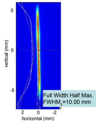
Figure 6: Streaked beam on the observation screen for “on crest” acceleration
