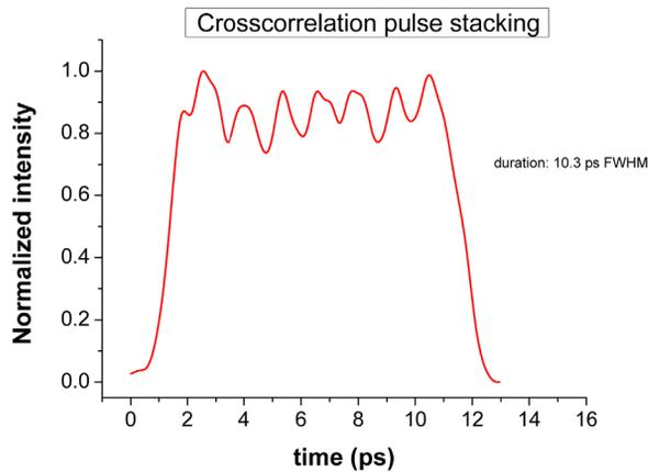
Figure 2: Measurement of the temporal profile of the UV laser pulse generated by pulse stacking.
