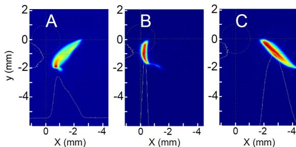
Figure 7: Streaked beam in the spectrometer arm (Vertical  $\propto$  Time, Horizontal  $\propto$  Energy). **A)** bunching mode +10 deg in first TW cavity, **B)** on crest, **C)** de-bunching mode -10 deg in first TW cavity.
