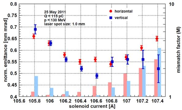
Figure 5: Emittance versus gun solenoid strength –after asymmetry correction via quad and skew quad integrated in the gun solenoid (115 pC, 130 MeV)
