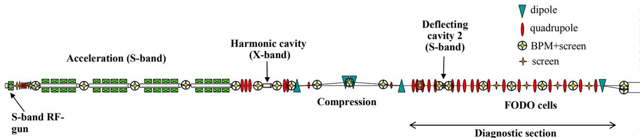
Figure 1: Schematic layout of the SwissFEL Injector Test Facility.
