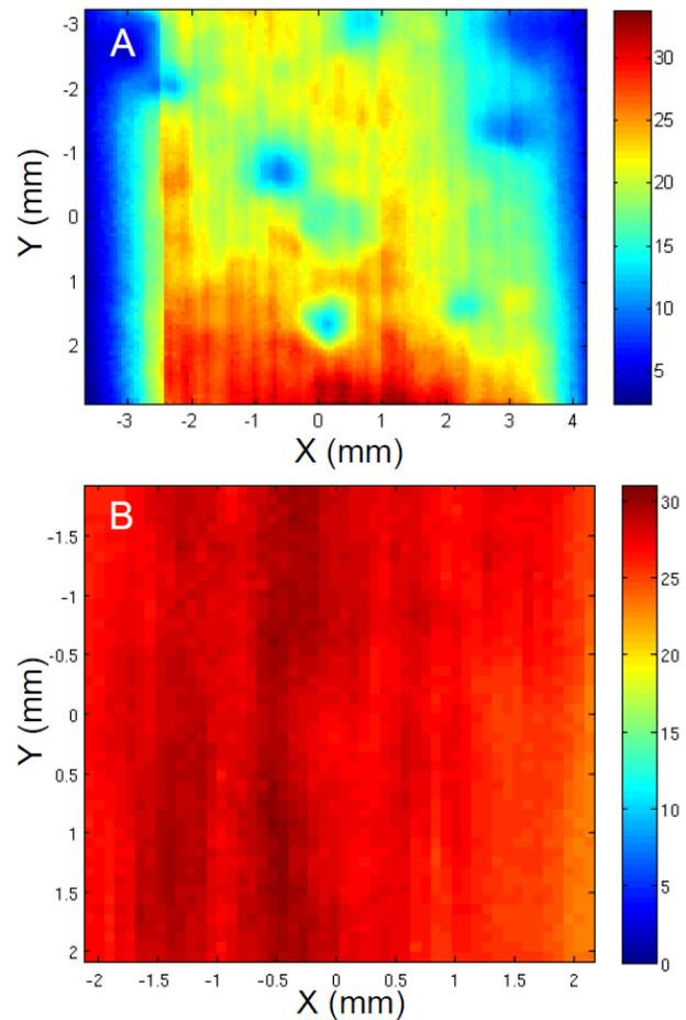
Figure 3: Cathode extracted charge - contour plot (a.u.). A) First cathode. B) Second cathode after installation
