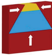
Figure 5: Magnet geometry for simulations. The red blocks are PrFeB magnets pointing to the transversally wedged pole. The blue block is made from CoFe, the brown one from CoFe or Dysprosium or Holmium.
