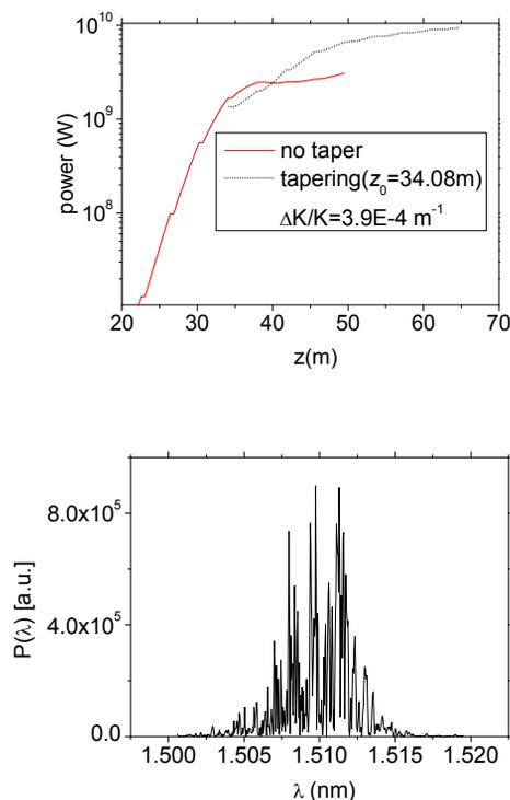
Figure 4: Tapering from the point near saturation ( $z_0=34.08$  m). **Top:** Radiation power curves with and without tapering. **Bottom:** Radiation spectrum at saturation of tapered FEL with tapered rate  $\Delta K/K = 3.9 \times 10^{-4} \text{ m}^{-1}$ .
