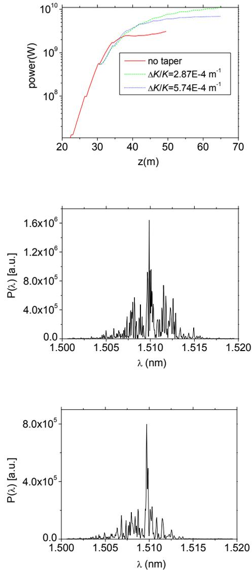
Figure 3: Tapering from the end of the exponential gain region ( $z_0=30.24 \text{ m}$ ). **Top:** Radiation power curves with and without tapering. **Middle:** Radiation spectrum at saturation of tapered FEL with tapered rate  $\Delta K / K = 2.87 \times 10^{-4} \text{ m}^{-1}$ . **Bottom:** Radiation spectrum at saturation of tapered FEL with tapered rate  $\Delta K / K = 5.74 \times 10^{-4} \text{ m}^{-1}$ .
