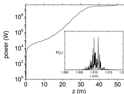
Figure 1: Radiation power of SASE FEL without tapering and the spectrum at saturation.
