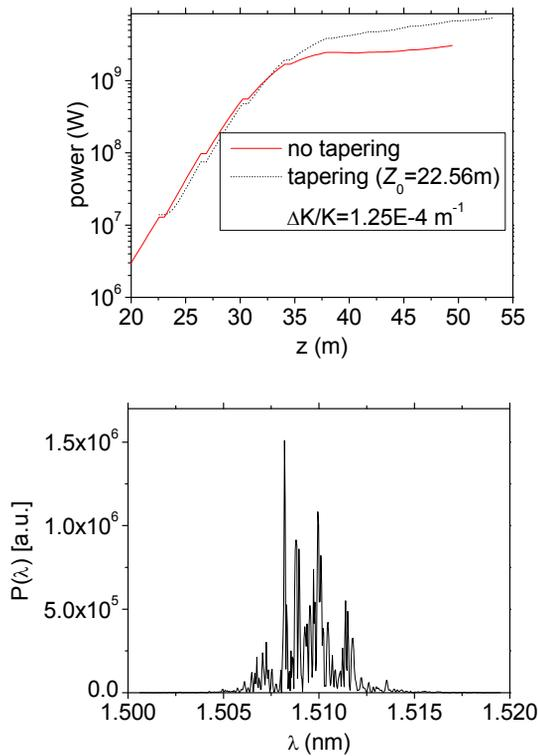
Figure 2: Tapering from the middle of the exponential gain region ( $z_0=22.56 \text{ m}$ ). **Top:** Radiation power curves with and without tapering. **Bottom:** Radiation spectrum at saturation of tapered FEL with tapered rate  $\Delta K / K = 1.25 \times 10^{-4} \text{ m}^{-1}$ .
