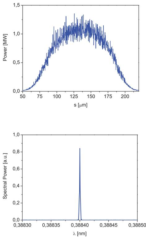
Figure 4: Output of the harmonic radiator of the combined FEL setup showing the power profile (top) and the spectral distribution (bottom).
