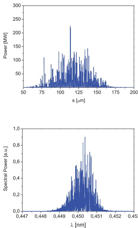
Figure 6: Output power of an ERL driven SASE-FEL utilizing the current enhancement scheme showing the power profile (top) and the spectral distribution (bottom).
