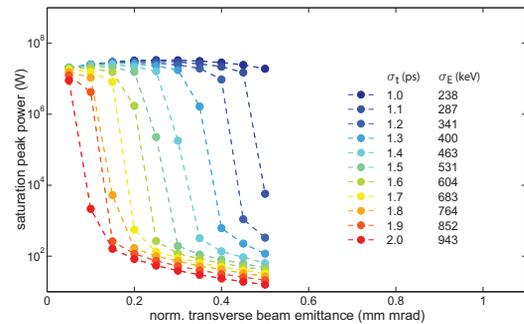
Figure 7: Calculated intra-cavity power of a hard x-ray FEL Oscillator driven by the Cornell ERL. Shown is the saturation peak power as a function of transverse beam emittance and bunch duration. A bunch charge of 25 pC is assumed, the undulator has 3000 periods with a period length of 15 mm. The radiation wavelength is 0.103 nm. We assume spectral losses on the order of 15% per roundtrip, including 4% out-coupled power.
