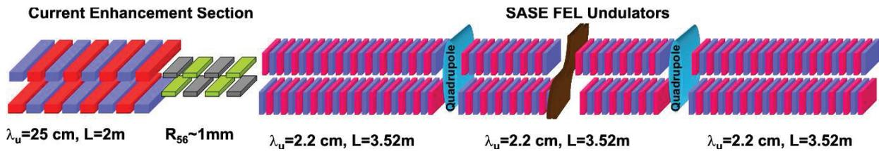
Figure 5: A SASE FEL setup for an ERL consisting of a current enhancement section and an undulator section. The current enhancement part consists of a 2 m long undulator with a period length of 25 cm and a chicane with an  $r_{56}$  of about 1 mm. The SASE FEL section consists of 12 undulators, each 3.52 m long with a period length of 2.2 cm.
