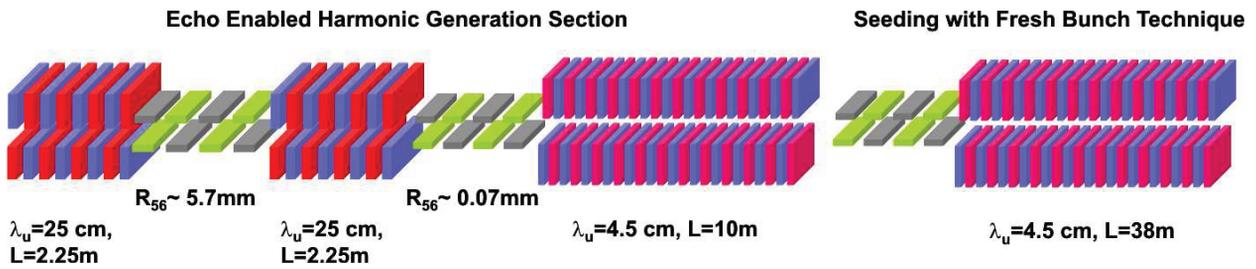
Figure 1: Using the fresh bunch technique [7], a radiator following a regular Echo enabled FEL [4] can deliver high power radiation pulses of soft x-rays. The EEHG part consists of two 2.25 m modulators, each with a period length of 25 cm. The EEHG-radiator has a period length of 4.5 cm and consist of two undulators each 4.5 m long. The second radiator consists of 8 undulators, each 4.5 m long with a period length of 4.5 cm.
