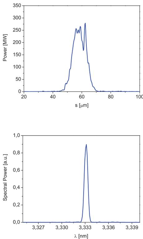
Figure 2: The final output of the combined FEL setup showing the power profile (top) and the spectral distribution (bottom).
