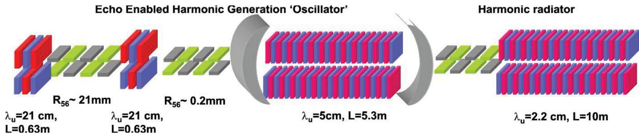
Figure 3: Using an oscillator as radiator following a regular Echo enabled modulation system [4] high power radiation can be delivered in hard x-rays range. The EEHG part consists of two 0.63 m modulators, each with a period length of 21 cm. The oscillator has a period length of 5 cm and is tuned to 2 nm. The second radiator consists of 5 undulators, each 3.52 m long with a period length of 2.2 cm.
