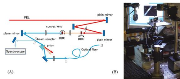
Figure 1: Schematic (A) and photo (B) of the microscopic irradiation system for VIS-FELs. The end of optical fibre (II) connects to the tapered-glass rod shown in (B). Details are described in the text.
