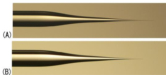
Figure 2: Tapered glass rods. (A) 5-µm tip, (B) 10-µm tip. Both rods were fabricated under the same conditions, and the cut was done at a diameter of 5-µm or 10-µm, respectively.
