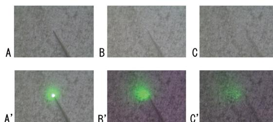
Figure 3: FEL (540 nm) power patterns at the tip of the fine-tapered glass rods. A and A', 0-mm from the tracing paper; B and B', 1-mm from the tracing paper; C and C', 2-mm from the tracing paper. Details are described in the text.
