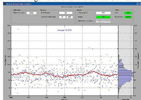
Figure 5: A 10 minutes continuous acquisition from the BAM station located downstream of BC1; each dot represents the rms value from 10 single shot acquisitions. The average value is 74fs.
