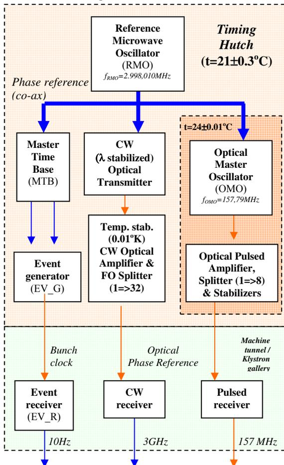
Figure 1: Basic block diagram of the FERMI@Elettra timing system. Blu lines indicate coaxial cables; orange lines, optical fibres. Temperature stability of the timing hutch and of individual systems is stabilized to 0.01°C.
