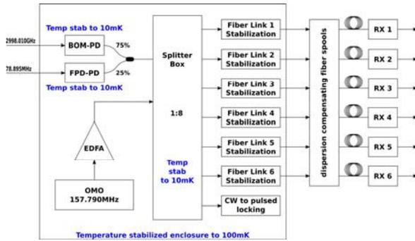
Figure 2: Pulsed optical timing system; the components, inside the box on the left, are temperature stabilized, down to 0.01°K.
