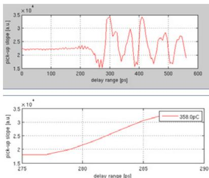
Figure 4: (Top) The BAM pick-up signal sampled by scanning the OMO pulse over it, with the optical delay line ( $\pm 300$ ps) fitted to the BAM Front-end. Bottom: the steep slope used for the calibration, assures a  $\pm 5$ ps linear window around the zero crossing, resulting in about 1200 counts /ps.
