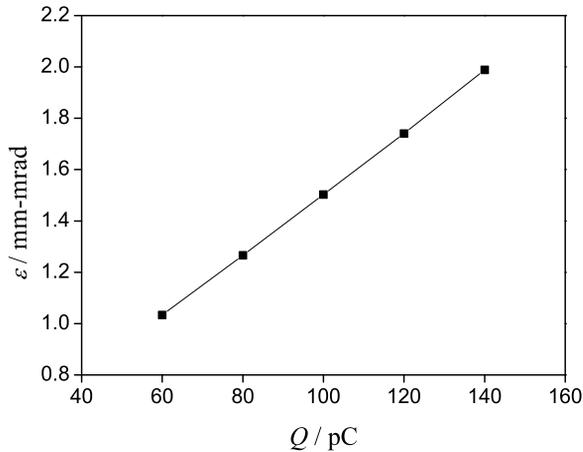
Figure 7: Minimal transverse emittances with different bunch charge.
