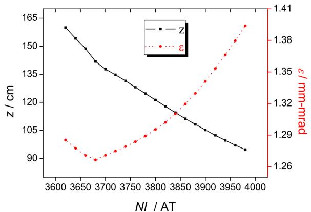
Figure 6: Minimal transverse emittances and positions with different solenoid current.
