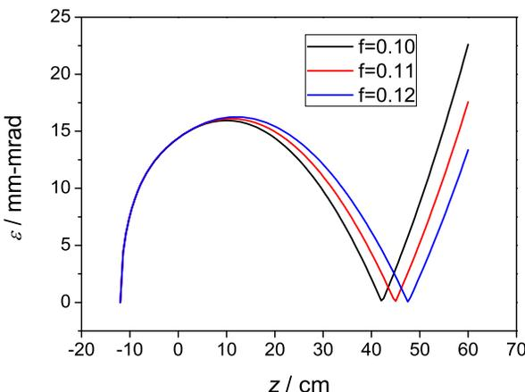
Figure 3: Transverse emittances with different solenoid focus length.
