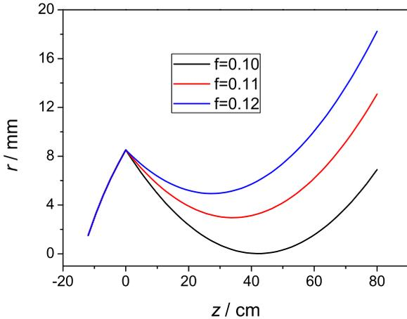
Figure 2: Beam radius with different solenoid focuslength.
