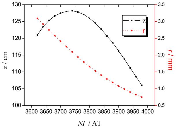
Figure 5: Minimal radius and positions with different solenoid current.
