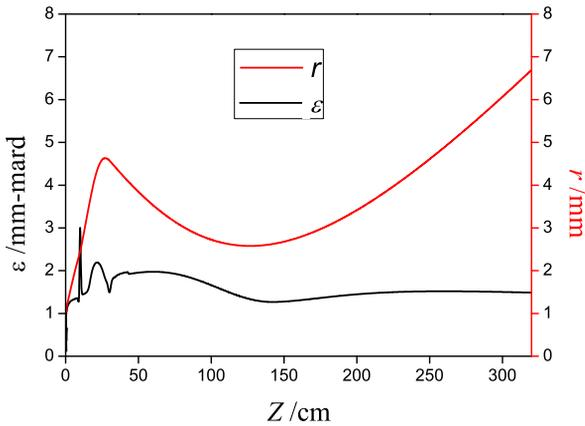
Figure 4: Results of solenoid compensation.
