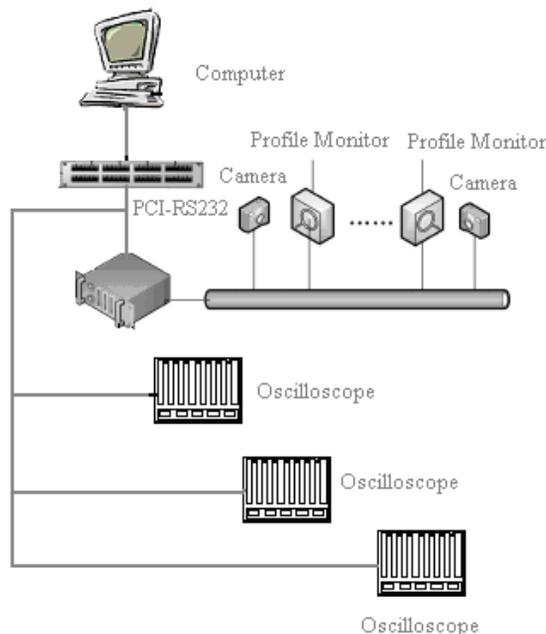
Figure 3: Architecture of Beam diagnostic system
