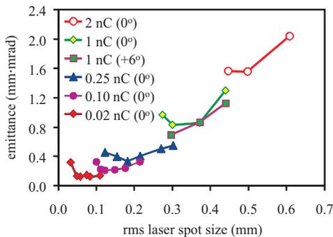
Figure 7: Measured geometric mean emittance ( $\varepsilon_{xy}$ ) as a function of the rms laser spot size for different bunch charges. All emittance values were analyzed from the 100% rms phase-space distribution.
