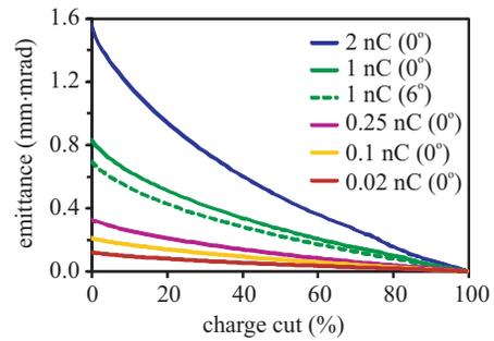
Figure 9: Geometric mean emittance ( $\varepsilon_{xy}$ ) as a function of charge cut for different bunch charges.
