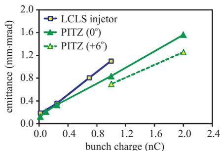
Figure 8: Comparison of measured geometric mean emittance ( $\varepsilon_{xy}$ ) as a function of the bunch charge for PITZ and LCLS injector beams.
