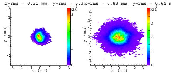
Figure 4: Transverse beam distribution on the YAG screens at EMSY1 (left) and at the beamlet observation station (right) for a bunch charge of 1 nC. The screens are located at 5.74 and 8.38 m downstream of the cathode, respectively.
