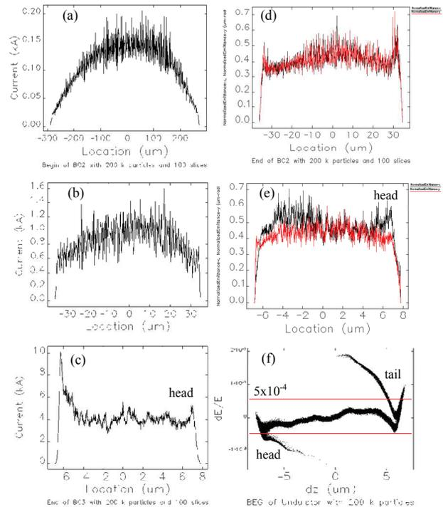
Figure 3: Start-to-End simulation result of the lattice: current profile (a) downstream BC1 and (b) downstream BC2, and (c) downstream BC3, and normalized emittance (d) downstream BC2 and (e) downstream BC3, and (f) longitudinal phase space before undulator. In (d) and (e), the black and red lines represent the horizontal and vertical emittances, respectively
