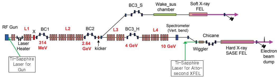
Figure 4: Layout of PAL XFEL. L1, L2, L3, and L4 represents S-band accelerating sections, BC3-S and BC3-H represent the 3rd bunch compressor for soft and hard X-ray beam line, respectively. Wake-sus-chamber represents a sus pipe chamber to introduce resistive wall wakefield.
