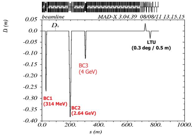
Figure 2: Dispersion function of the lattice. LTU represents the linac to undulator line consisting of four dipoles with the bend angle of 0.3 degrees.
