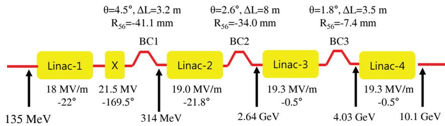
Figure 1: Three bunch compressor lattice for PAL XFEL. BC1, BC2, and BC3 represent the four-dipole chicane-type bunch compressors.  $\Delta L$  represents the distance between the first and the second dipoles of chicane.
