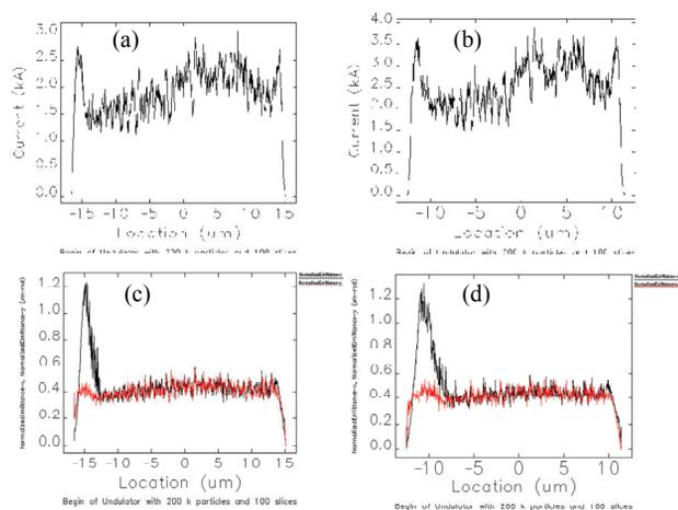
Figure 5: 2.64-GeV / 0.2 nC electron beam properties at the entrance of undulator for soft X-ray beamline: (a) and (b) bunch currents at different bend angles of BC3-S, and (c) and (d) are the corresponding normalized emittances to (a) and (b).
