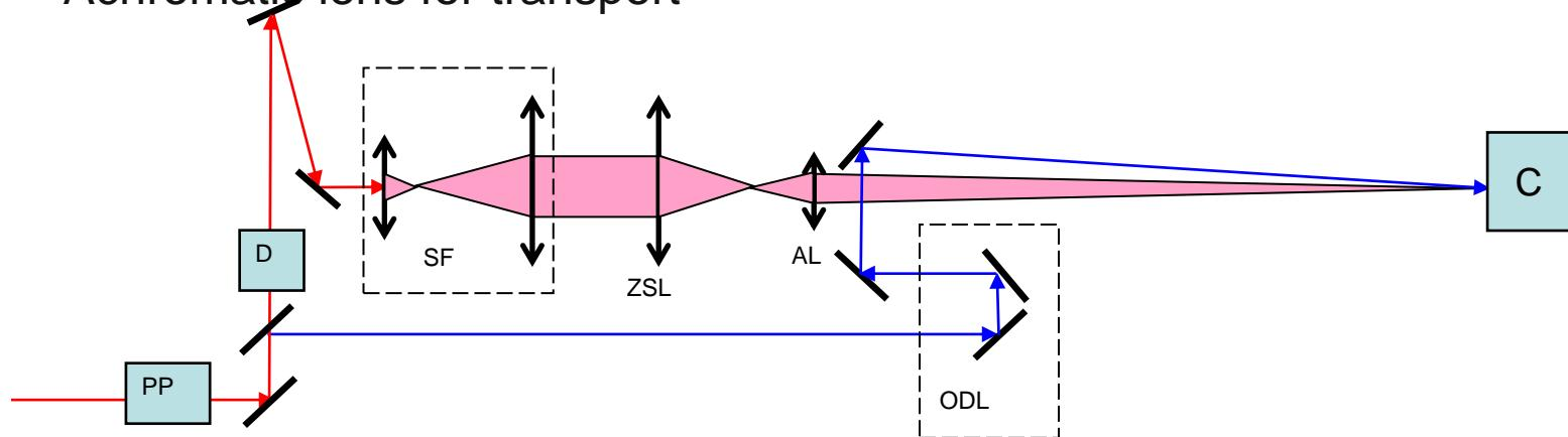
PP: pulse picker; D: AOPDF; SF: achromatic spatial filter; ZSL: ZnSe lens; AL: achromatic image relay lens; ODL: optical delay line; C: camera.
