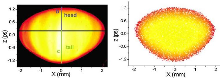
FIG. 5 (color online). Measured (left) and simulated (right) asymmetric beam distribution for  $Q = 50$  pC.
