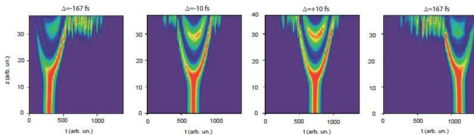
1 GeV e- beam. Seed: 300 kW @ 8.9 nm. 200xU26 – R<sub>56</sub> – 500xU26.
