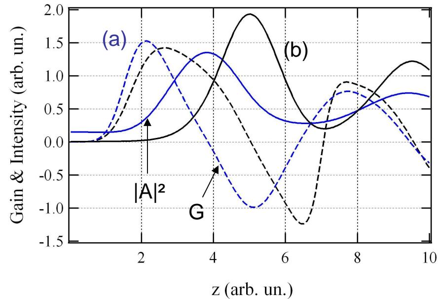
Local gain → Local saturation → Progressive saturation along the pulse
