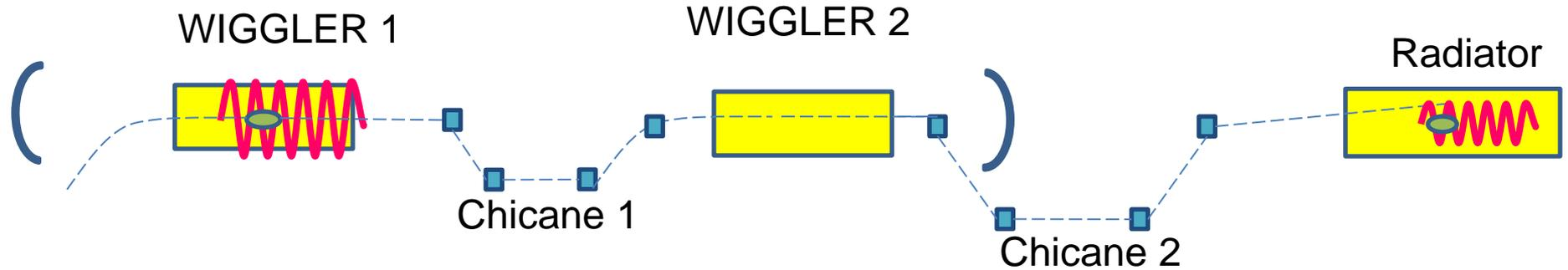
Chicane 1 acts to reduce bunching and lower intracavity power
