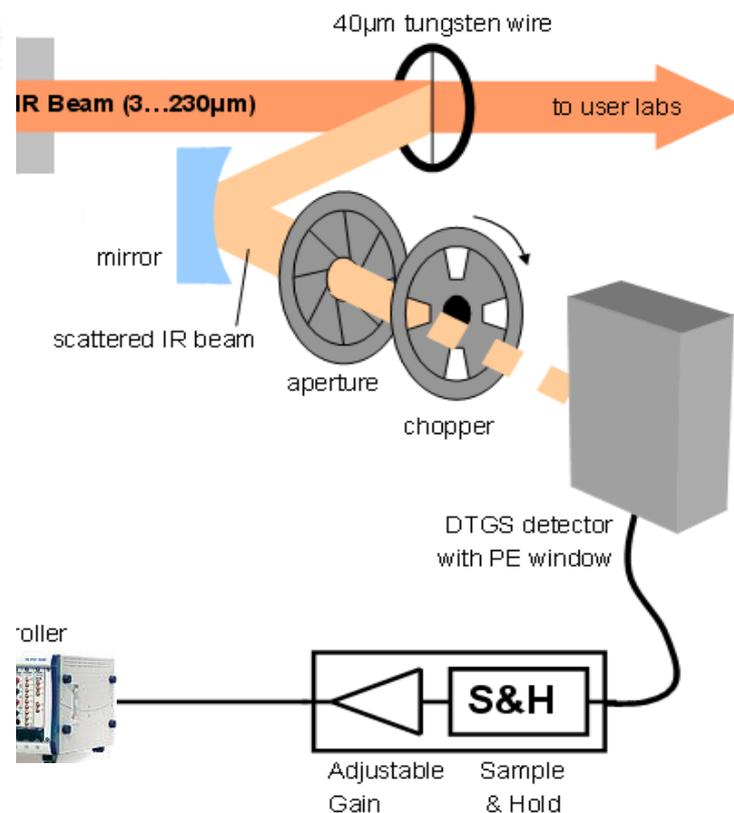
Test with chopper frequency of 2.4 kHz brought an improvement of only ~ 6dB @ 50 Hz due to limitation of the chopper phase stability and the DTGS rise time
