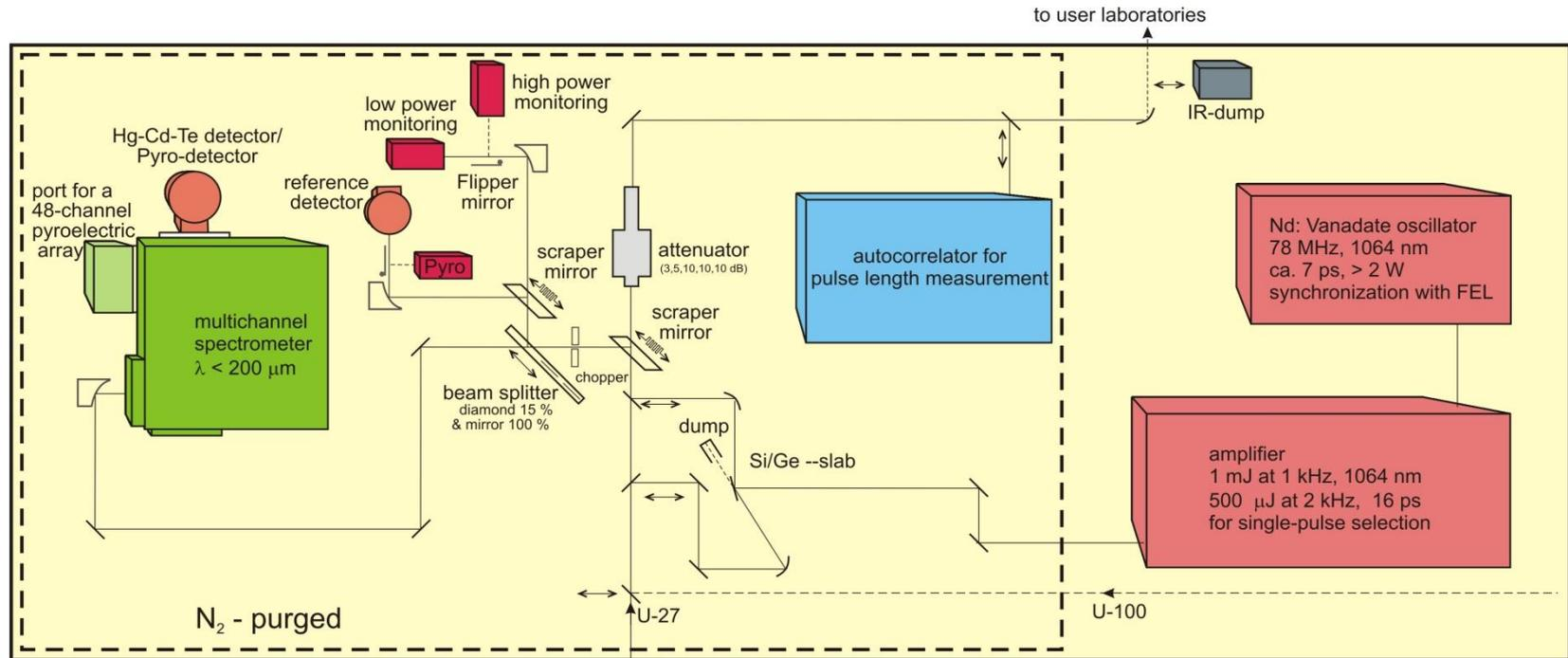
Interface of the remote controlled part of the diagnostic station
