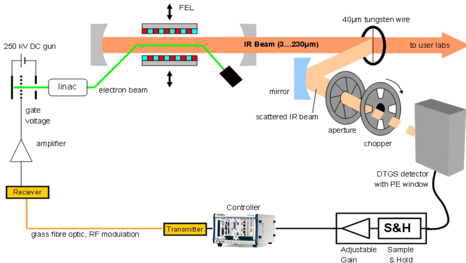
Test with chopper frequency of 2.4 kHz brought an improvement of only ~ 6dB @ 50 Hz due to limitation of the chopper phase stability and the DTGS rise time
