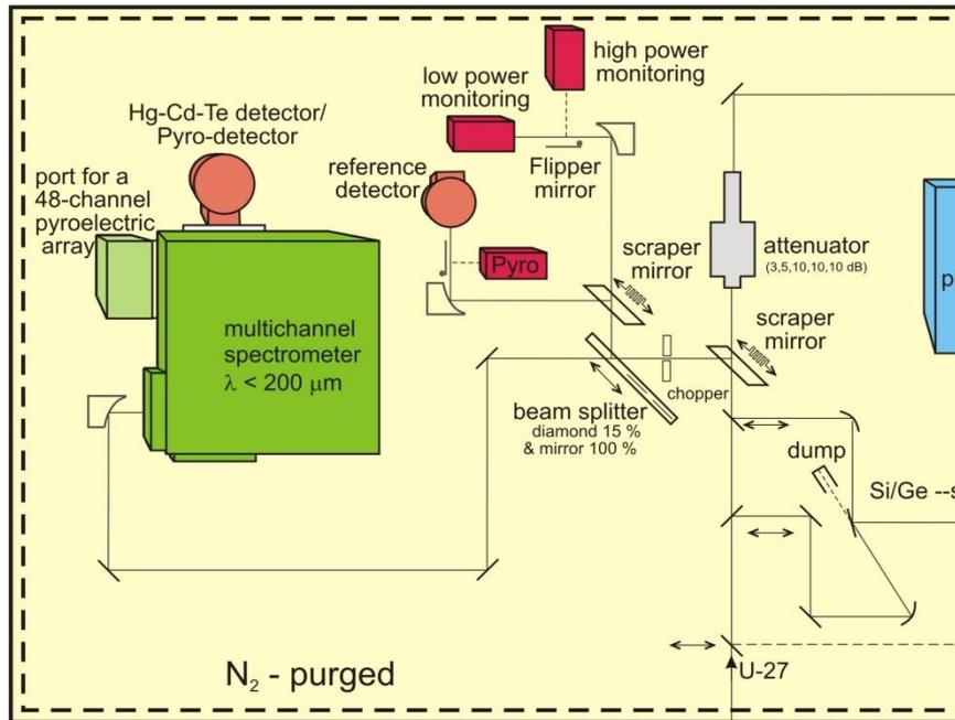
Interface of the remote controlled part of the diagnostic station
