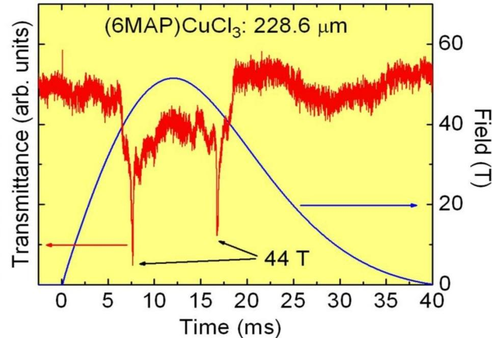
No synchronization of the FEL with the magnetic pulses is needed, since the FEL runs continuously at 13 MHz > 10<sup>6</sup> FEL pulses during one magnetic-field pulse of 100 ms length provide excellent measurement conditions
