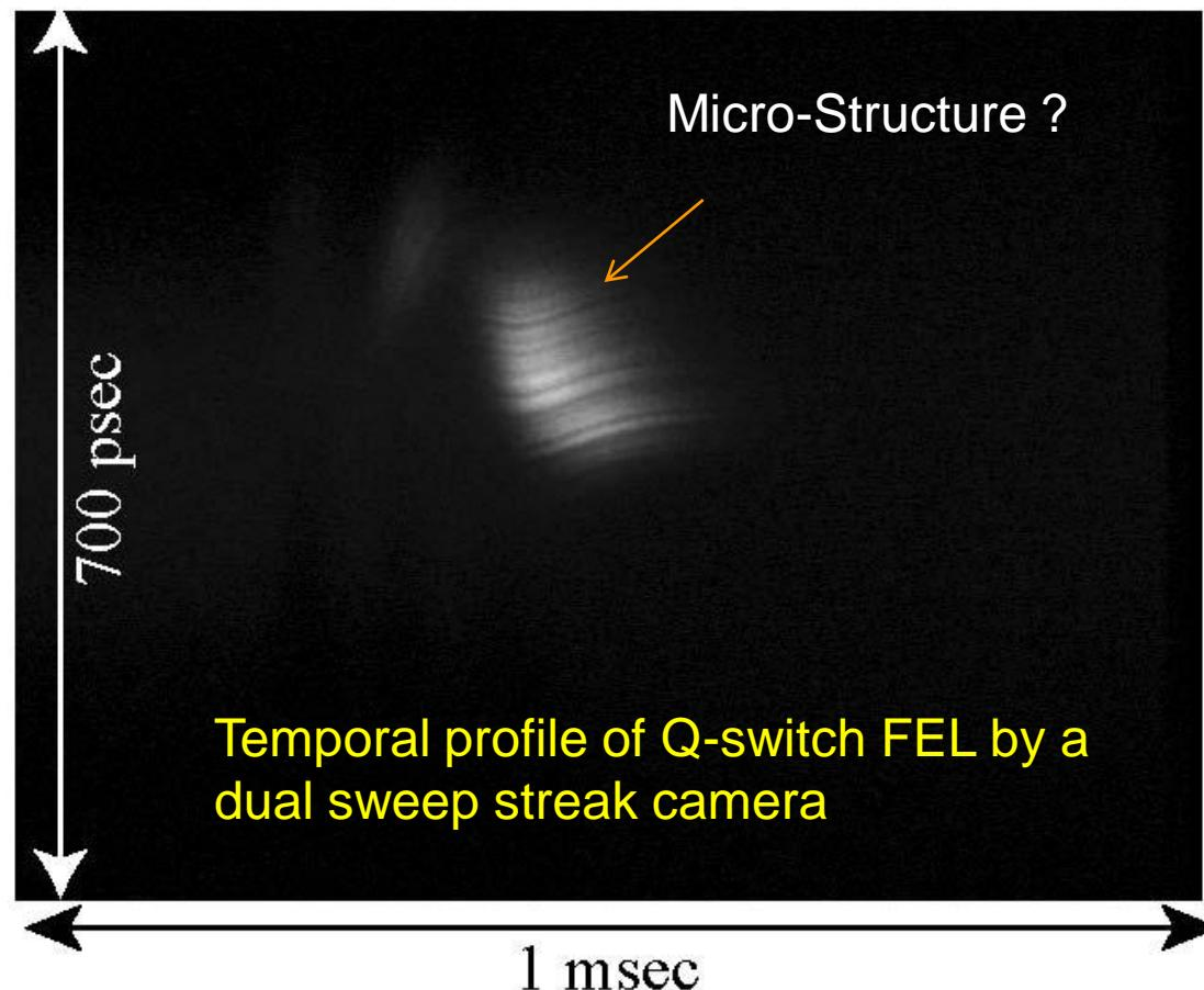
Sub-picosecond Micro-structure in Q-switch FEL Pulse?
