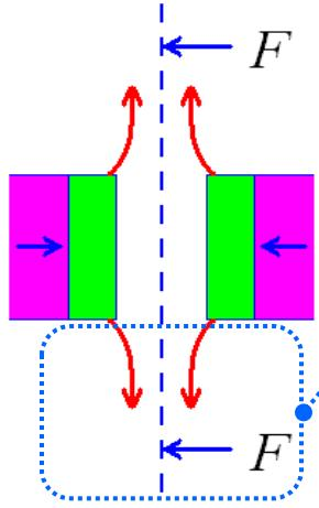
The force is caused by magnetic field pressure
