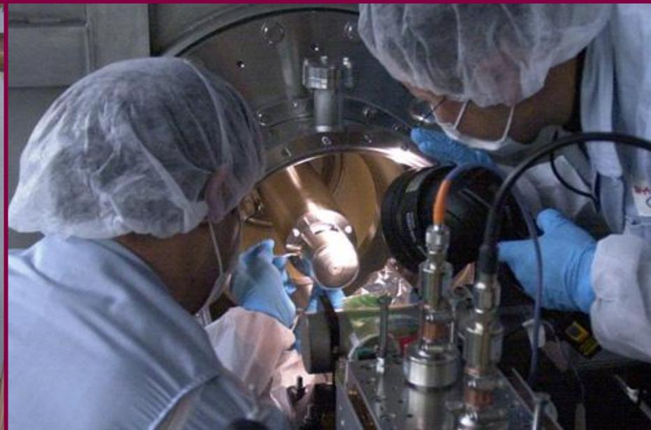
We replaced CeB6 crystal in SCSS accelerator, after 20,000 hour operation.
