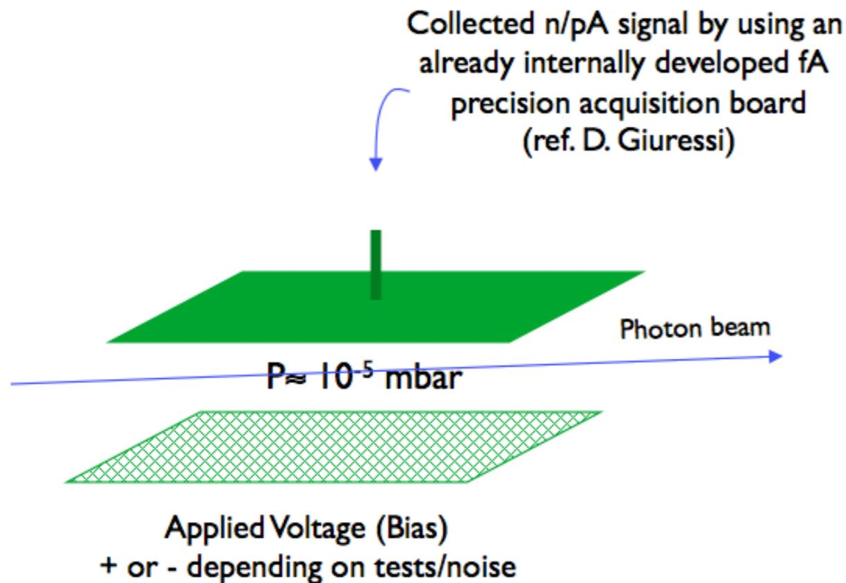
Calibrated with High precision IRD photodiodes
