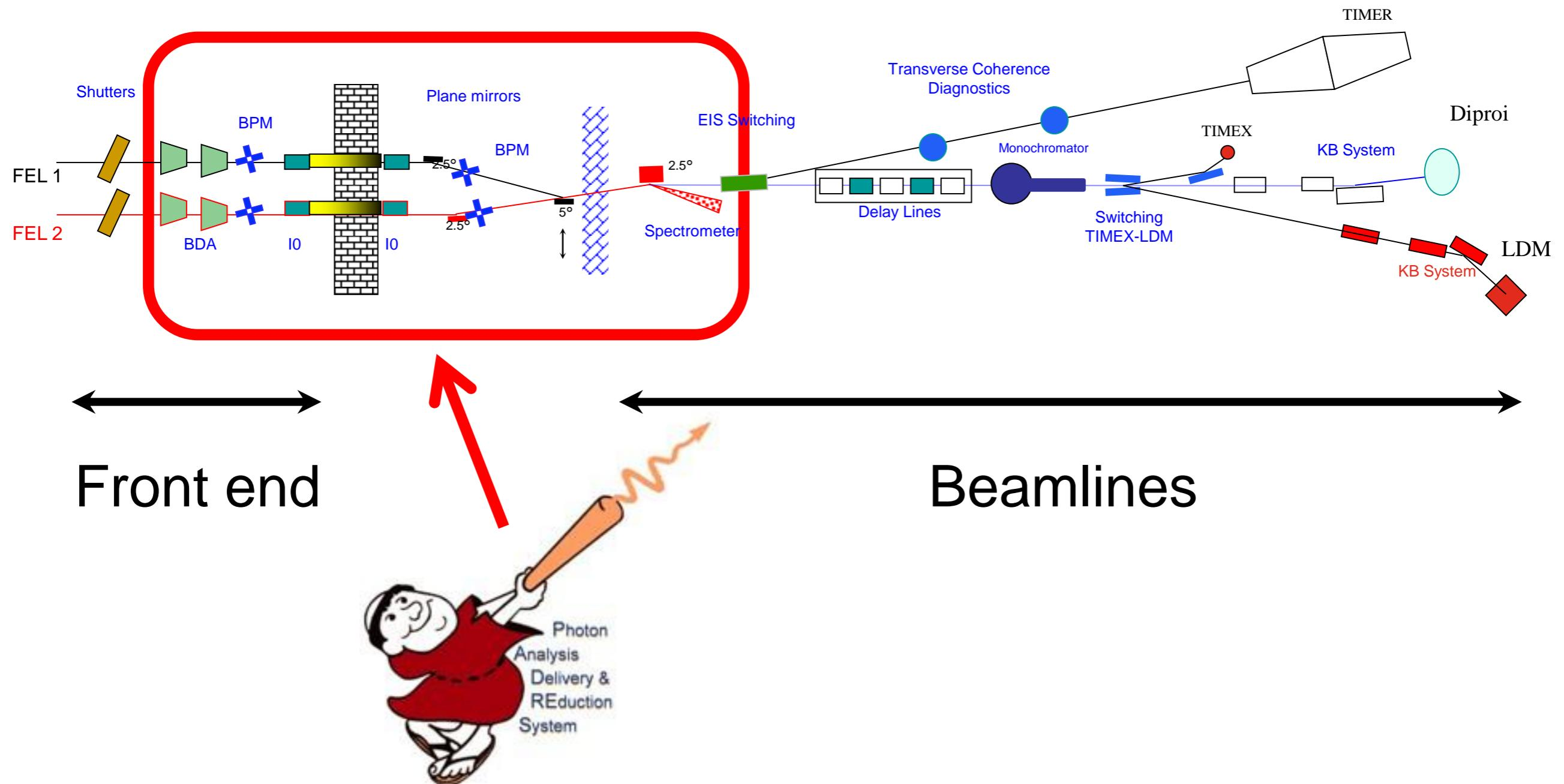
**Target:** collect both FEL paths, diagnose, and redirect to the beamlines
