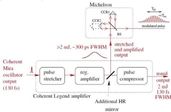
Figure 5. Laser pulse shaper to produce amplitude modulated pulses [25].
