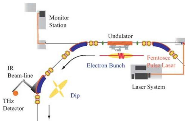
Figure 2: Layout of the laser modulation system at UVSOR-II. A part of the storage ring of 53 m circumference is shown [16].
