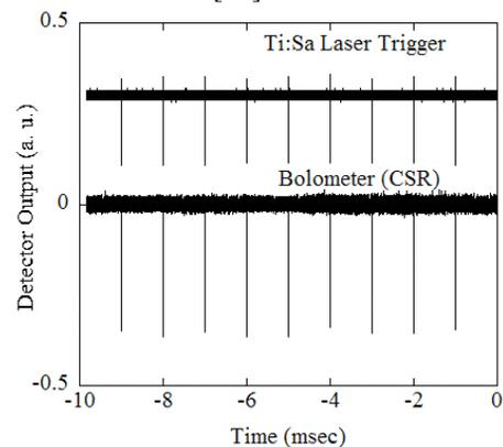
Figure 3: Laser injection timing and bolometer output. Between the intense THz emission of 1 kHz repetition, normal synchrotron radiation is continuously emitted but in the background [16].
