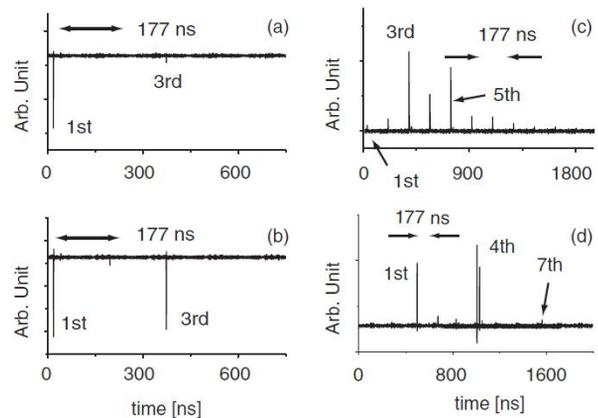
Figure 7. CSR observed turn-by-turn in the low-alpha mode [27]. Revolution time of the ring is 177 ns. (a)-(c) are for the betatron tune close to a half integer. Sensitivity ranges are (a) 11.0-16.6 cm<sup>-1</sup>, (b) 7.3-11.0 cm<sup>-1</sup>, and (c) 3.7-5.7 cm<sup>-1</sup>. (d) is for the betatron tune close to one third of an integer. Sensitivity range is same as (c).
