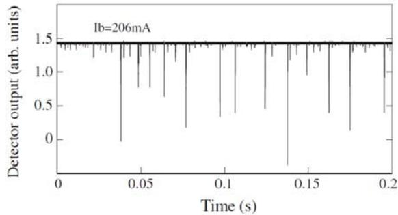
Figure 1: THz bursts observed at UVSOR-II in the single bunch operation mode. The observed wavelength is in the range of 0.2 – 3 mm. [12]
