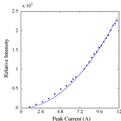
Figure 4: CSR intensity versus peak current of electron bunch [16].
