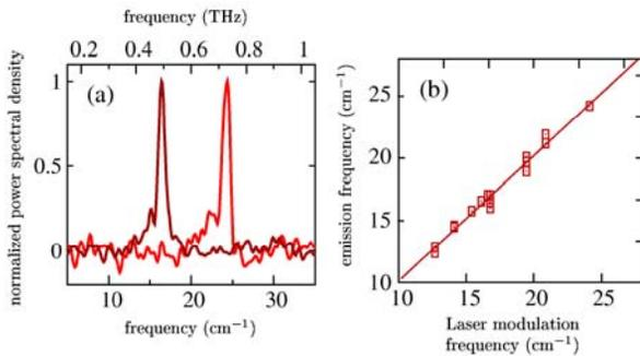
Figure 6. Monochromatic and tunable CSR produced by laser modulation technique [24]. Left: Examples of observed spectra. Right: Correlation between the laser modulation frequency and the THz emission frequency.
