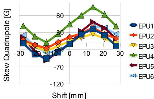
Figure 6: Shift dependent skew quadrupole at 22 mm gap. The dependency is present in all EPUs. Origin of this skew quadrupole is unknown, most probably due to micro movements as discussed in [3].
