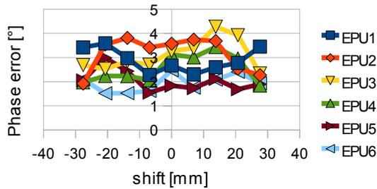
Figure 4: Shift dependency of phase error at 22 mm gap for all EPUs. Phase Error is within the specified limit of  $5^\circ$ . Just in three undulators it was necessary to compensate the shift dependency by dynamic tapering.
