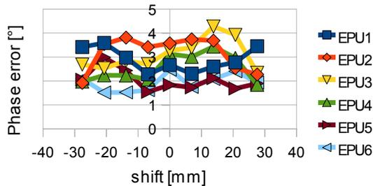
Figure 4: Shift dependency of phase error at 22 mm gap for all EPU. Phase Error is within the specified limit of  $5^\circ$ . Just in three undulators it was necessary to compensate the shift dependency by dynamic tapering.
