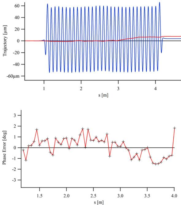
Figure 2: LPU Modulator; Electron beam trajectory and phase error at 1.2 GeV electron beam energy. Trajectory straightness is within 4 micrometers and phase error is  $0.87^\circ$ .
