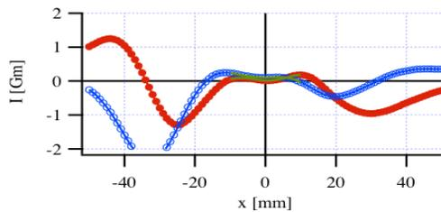
Figure 5: EPU #6 integrated field integrals at 0 shift and 10 mm gap. Normal field integral (blue) and skew field integral (red) are shown.
