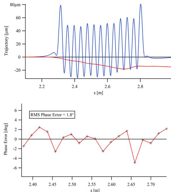
Figure 1: Laser Heater Undulator electron beam trajectory and phase error at 24 mm gap. RMS phase error is 1.8°. Trajectory straightness is within 6 micrometers. Electron beam energy is 100 MeV.
