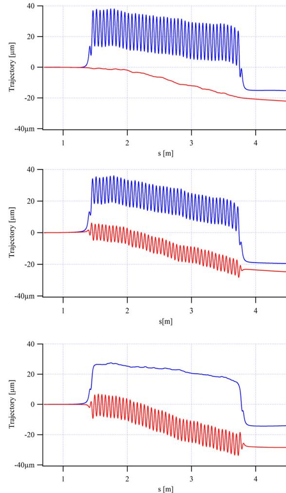
Figure 3: Electron beam trajectory for EPU 3 at 20 mm gap, for 0, 1/4 and 1/2 period shifts (top down). This trajectory was achieved by assembly optimization only, without any shimming. Vertical trajectory (red) and horizontal electron trajectories (blue) are shown.
