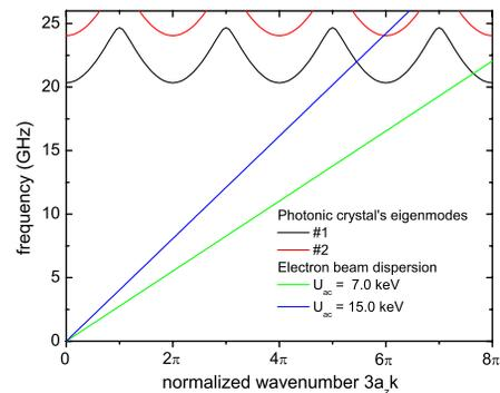
Figure 4: Dispersion of the first two TM-like modes of the PhC and electron beam dispersion for beam energies of  $U_a = 7$  keV and  $U_a = 15$  keV.
