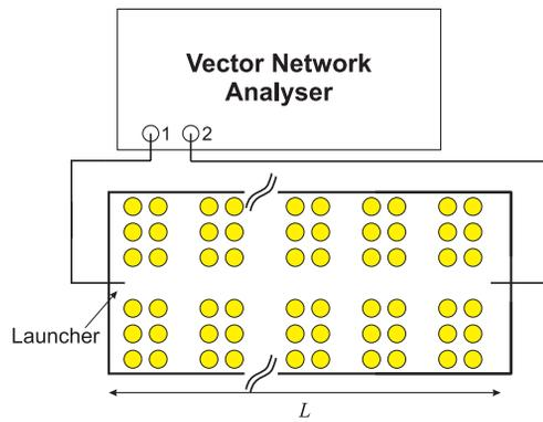
Figure 5: Experimental setup to verify the dispersion of the PhC: A Vector Network Analyser excites by a launcher a cavity of 15 unit cells of the PhC, a similar launcher at the end acts as a receiver.
