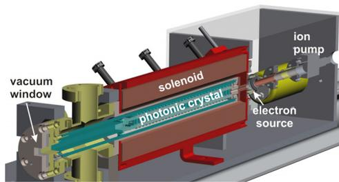
Figure 2: 3 dimensional drawing of the spFEL setup.
