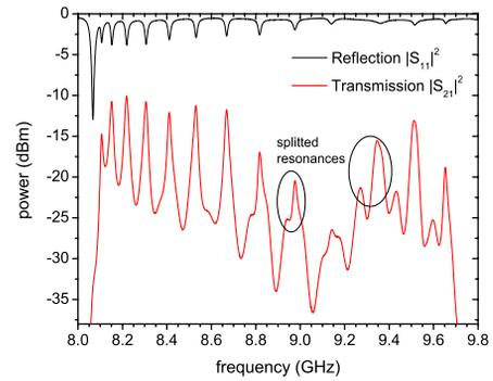
Figure 6: Measured transmission and reflection spectrum from the setup shown in Fig.5.
