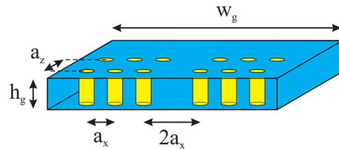
Figure 3: Unit cell of the PhC for the single beam pFEL, consisting of a rectangular waveguide and metal posts of radius  $r = 0.75$  mm,  $a_x = 2.7$  mm,  $a_z = 3$  mm,  $w_g = 18.9$  mm,  $h_g = 8$  mm.
