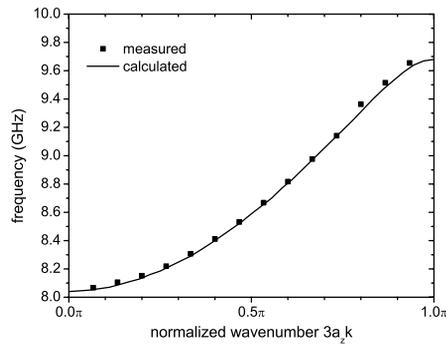
Figure 7: Comparison between measured and calculated dispersion of the lowest TM-like PhC mode.
