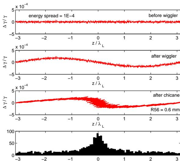
Figure 5: Micro-bunching by laser modulation. The first graph is relative energy spread for one laser wavelength before wiggler, the second after wiggler, the third after chicane, and the last is the electron distributions after chicane.
