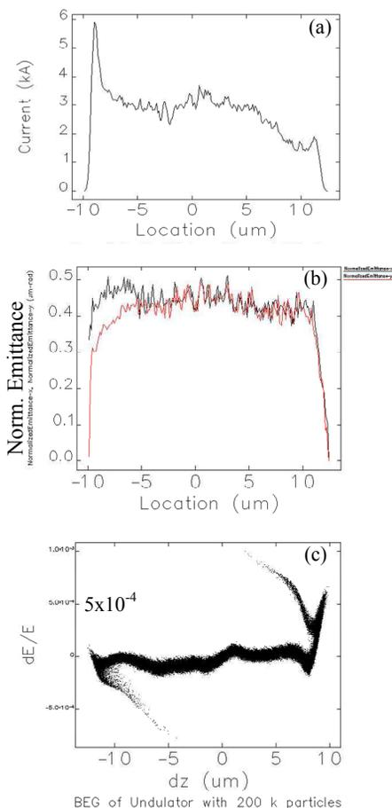
Figure 2: 10-GeV / 0.2 nC electron beam properties at the entrance of undulator: (a) current profile, (b) normalized emittance, and (c) longitudinal phase space. In (b) the black and red lines represent the horizontal and vertical emittances, respectively.
