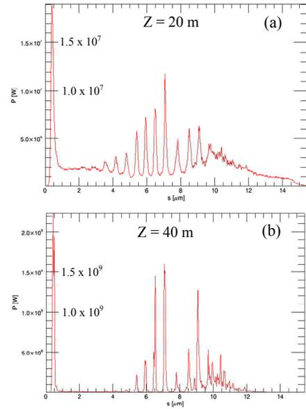
Figure 7: 0.1 nm SASE output at two different location of undulator: (a) 20 m, (b) 40 m.
