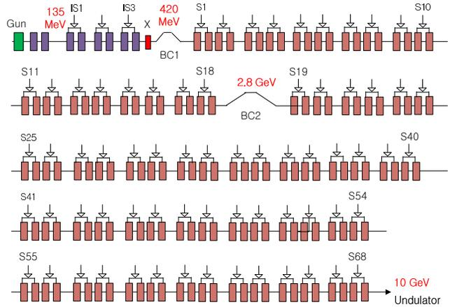
Figure 1: Layout of PAL-XFEL. BC1 and BC2 represent first and second chicane-type bunch compressor.
