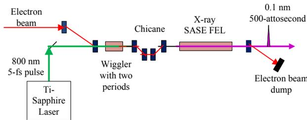
Figure 4: ESASE Scheme for atto-second XFEL radiation.
