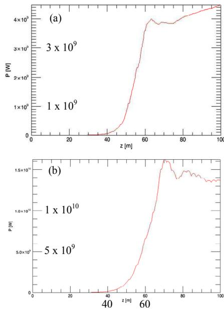
Figure 3: Genesis code simulation result for (a) 0.1 nm FEL and (b) 0.06 nm FEL. The electron beam energy is 10 GeV, and the beam charge is 0.2 nC.
