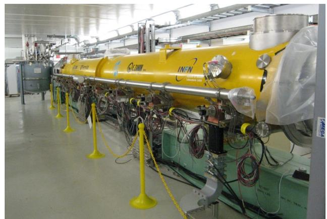
Fig. 4: Cryomodule 1 of type TTF III+ from DESY has been installed on its girder in the NML facility and commissioning will proceed in the coming months.
