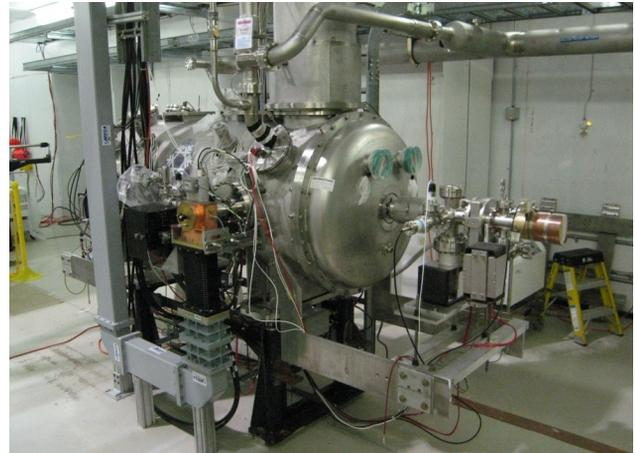
Fig. 3. Booster cavity 2 (from DESY and Saclay) has been installed in the NML facility and has a gradient of 24 MV/m.
