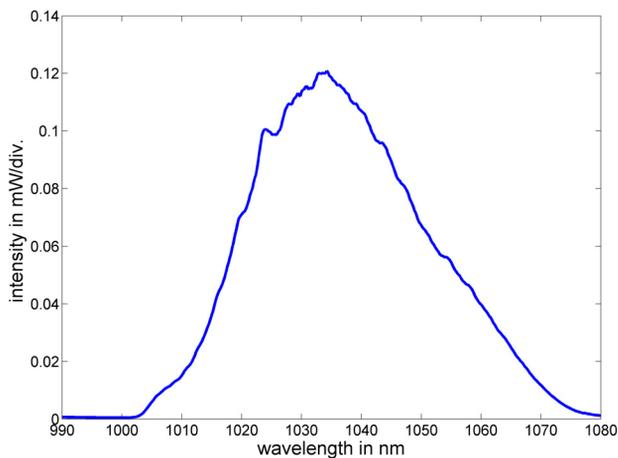
Figure 4: Optical spectrum of pre-amplified laser pulses.
