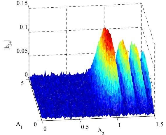
Figure 1: The bunching factor as a function of the two energy modulation parameters  $A_1$  and  $A_2$ .
