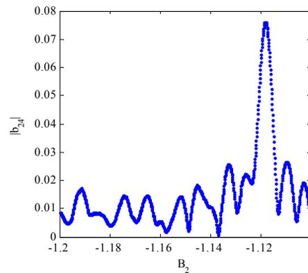
Figure 9: Bunching degradation due to an initial energy chirp can be compensated for by adjusting parameter  $B_2$  (from  $-1.14$  to  $-1.118$ ).
