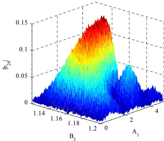
Figure 3: The bunching factor as a function of the first energy modulation parameter  $A_1$  and the second dispersive parameter  $B_2$ .
