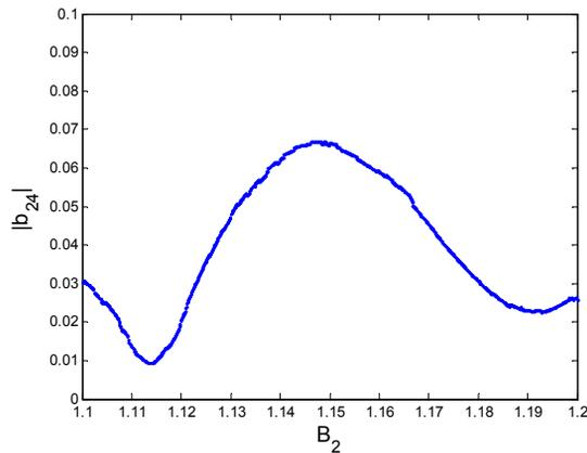
Figure 10: Bunching factor variation with  $B_2$  for the case of positive dispersive parameters,  $B_1$  and  $B_2$ .
