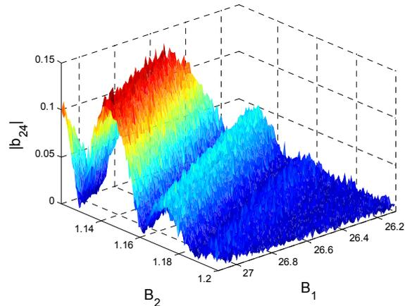
Figure 6: The bunching factor as a function of the first dispersive parameter  $B_1$  and the second dispersive parameter  $B_2$ .
