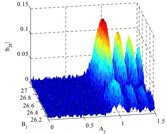
Figure 5: The bunching factor as a function of the second energy modulation parameter  $A_2$  and the first dispersive parameter  $B_1$ .
