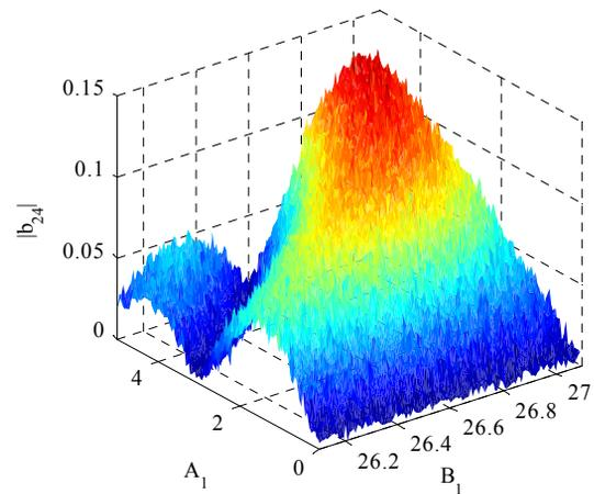
Figure 2: The bunching factor as a function of the first energy modulation parameter  $A_1$  and the first dispersive parameter  $B_1$ .
