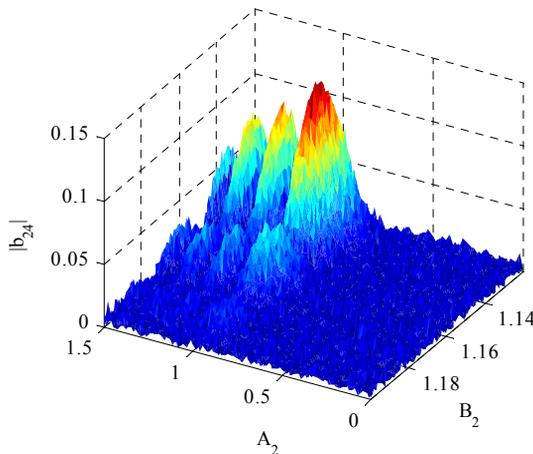
Figure 4: The bunching factor a function of the second energy modulation parameter  $A_2$  and the second dispersive parameter  $B_2$ .
