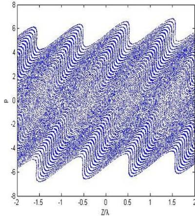
Figure 7: The second undulator and dispersive section generates a large density modulation at the harmonic in the beam's longitudinal plane.
