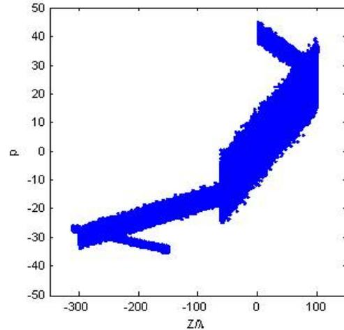
Figure 8: Approximation of a realistic electron beam distribution with non-linear energy chirp, based on [7].
